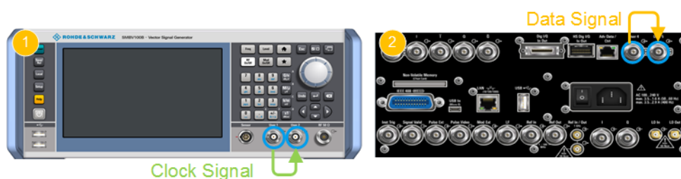
Figure 2-6: Looping back of the clock and data signals (the BER Data Enable signal is routed internally)
