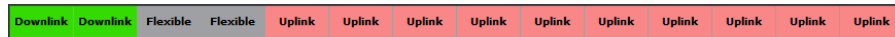
Figure 4-6: Preview of symbol usage for slot format 38 as defined in 3GPP 38.211, table 4.3.2-3
