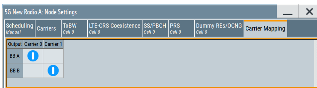
Figure 5-1: Carrier mapping of two carriers in a 2x1x1 coupled system
