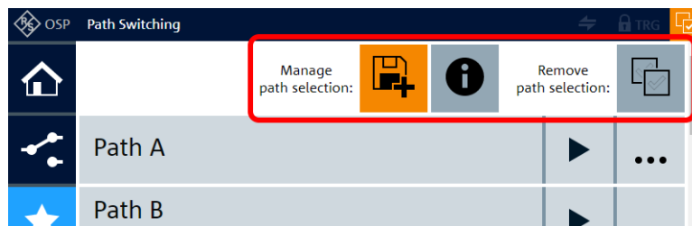
Figure 6-35: Path Switching dialog with existing paths and option for saving a new path
