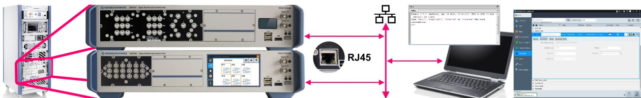
Figure 3-15: Remote operation by SCPI commands
