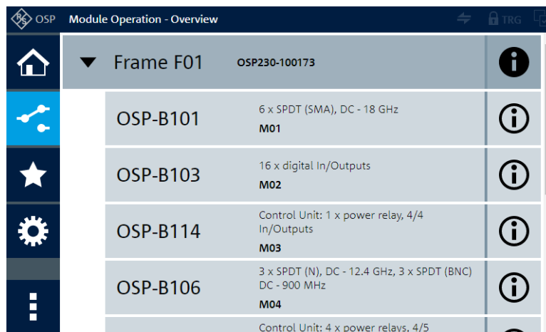
Figure 3-2: The module operation dialog, here with a single switch unit and 5 modules
