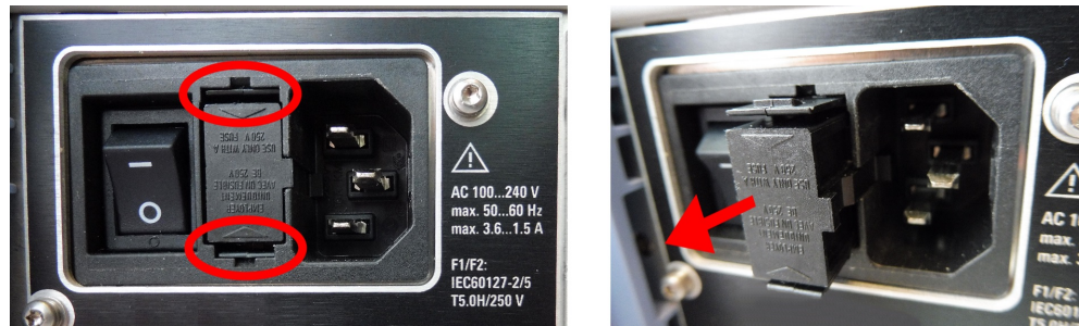
Figure 13-1: Removing the fuse holder (holes to unlock marked red)
