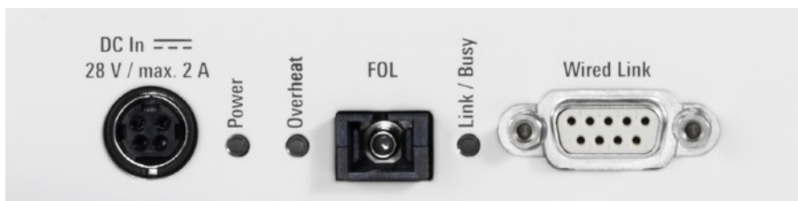
Figure 4-151: Connectors and LEDs on the rear panel of the R&S OSP-B200S2
