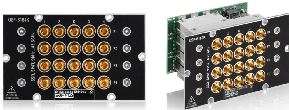
Figure 4-140: R&S OSP-B164K, here model .44 with four relays
