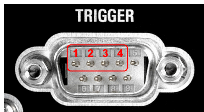
Figure 6-58: Pins 1 to 4 are the first 4 pins (left to right) in the top row of the male D-Sub 9 connector on the rear of the R&S OSP320. For allowable input voltage levels, refer to the specifications.
