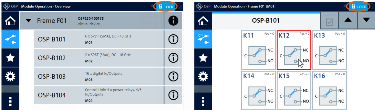
Figure 6-24: Module Operation dialog of a switch unit and of one module in lock mode
