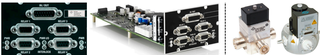
Figure 4-25: R&S OSP-B104 (detail on the right: 3rd-party Spinner relays)
