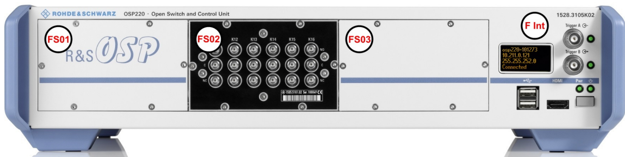
Figure 3-3: Front view of the R&S OSP220 (2HU)
