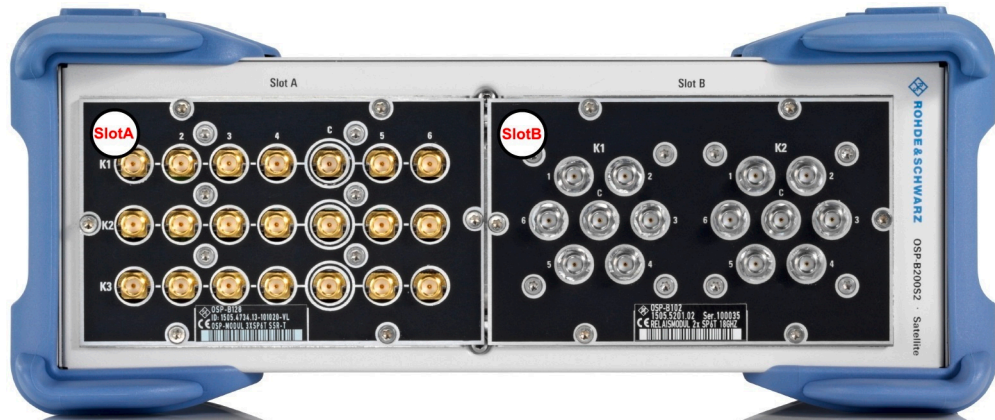
Figure 3-6: Front view of the R&S OSP-B200S2 (2HU)
