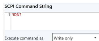
Figure 4-168: Example for the Identification command of a generic amplifier (here: from manufacturer "Bonn", which is shown as an editable Required Substring in Answer)
