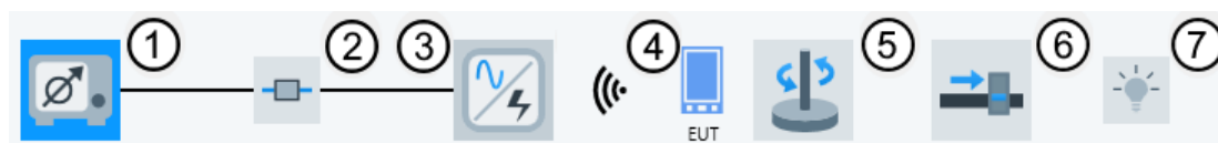
Figure 4-143: EMI radiated hardware setup diagram Magnetic Field Strength (Loop Antenna + Turntable)
