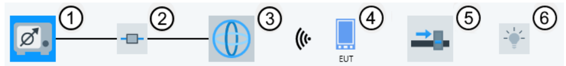
Figure 4-140: EMI radiated hardware setup diagram Magnetic Field Strength (Triple Loop Antenna)
