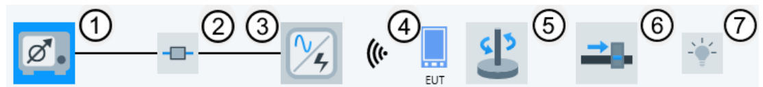
Figure 4-141: EMI radiated hardware setup diagram Magnetic Field Strength (Loop Antenna + Turntable)
