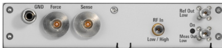
Figure 3-15: Connector side panel
