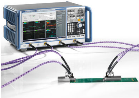
Figure 4-12: Test setup for fixture deembedding
