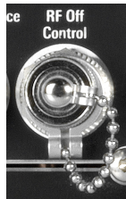
Figure 3-2: RF Off Control, terminated with attached Short
