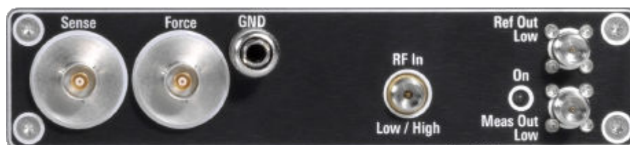
Figure 3-15: Connector panel of R&S ZVA-ZD110 Var 18 (system variants 02 to 07)
