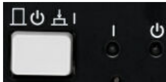
Figure 3-14: Standby switch and LEDs
