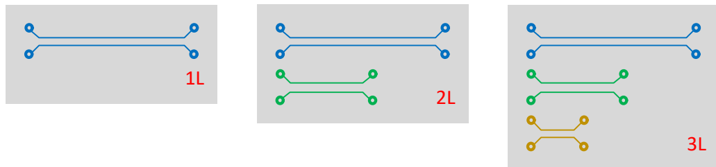
Figure 4-38: Test coupons for 1L, 2L and 3L measurements
