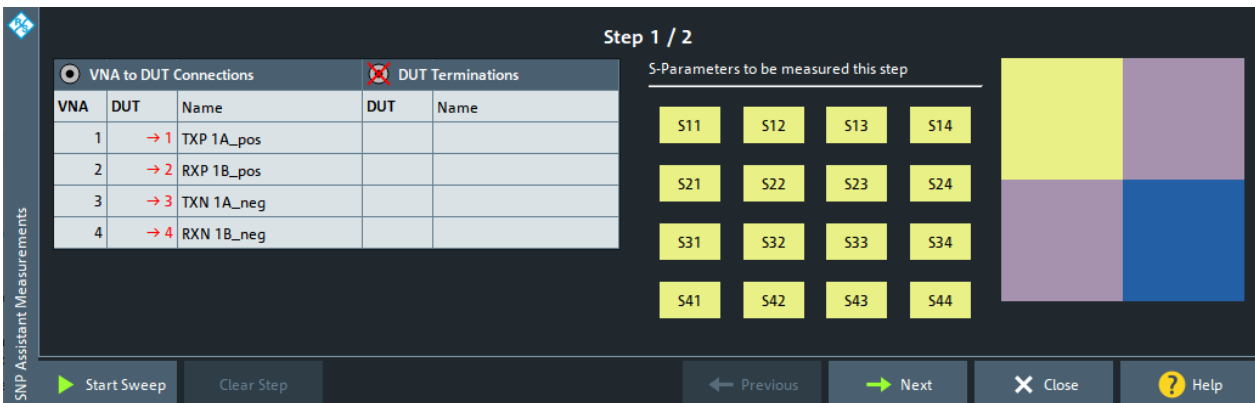
Figure 4-35: Step 3: Measure and/or import S-parameter data
