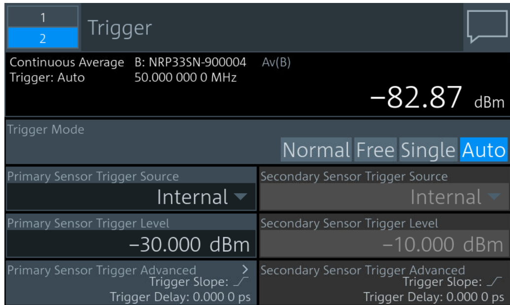
Figure 6-3: Display dialog, example for continuous average measurement
