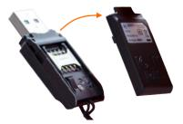
3. Insert the smart card with the chip facing downwards, and the angled corner (orange circle) facing away from the USB dongle:
