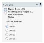
Figure 7-7: Accessories dialog for LISN control, here for a 4-line LISN
