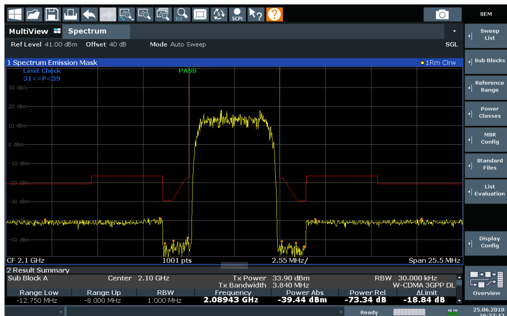
Figure 6-26: Detected peak display in SEM measurement
