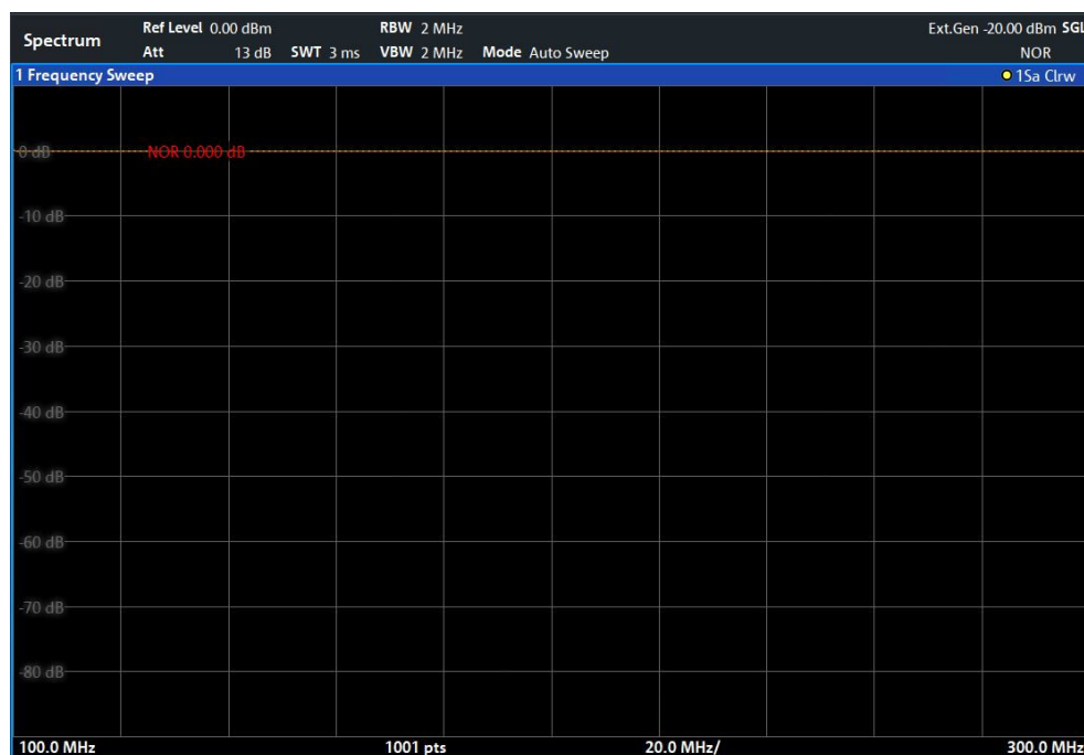
Figure 6-48: Normalized measurement results after calibration
