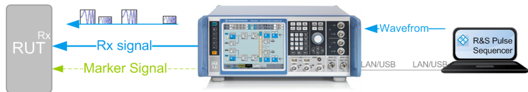
Figure 2-3: Radar echo generation with R&S SMW200A and ARB radar signals created by R&S Pulse Sequencer
