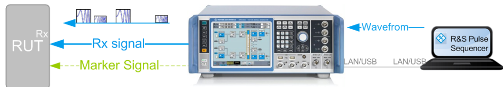
Figure 2-3: Radar echo generation with R&S SMW and ARB-based radar signals created by R&S Pulse Sequencer
