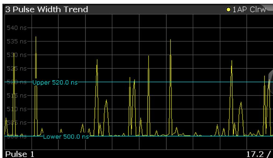
Figure 3-3: Pulse width trend display (over pulse numbers)
