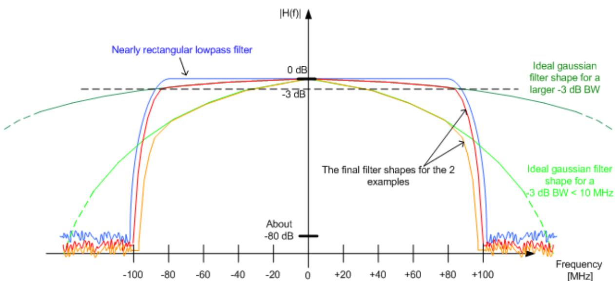
Table A-3: Gauss filters with large bandwidths (with R&amp;S FPS-B160)
