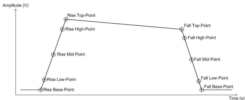
**Figure 3-2: Envelope model parameters**
