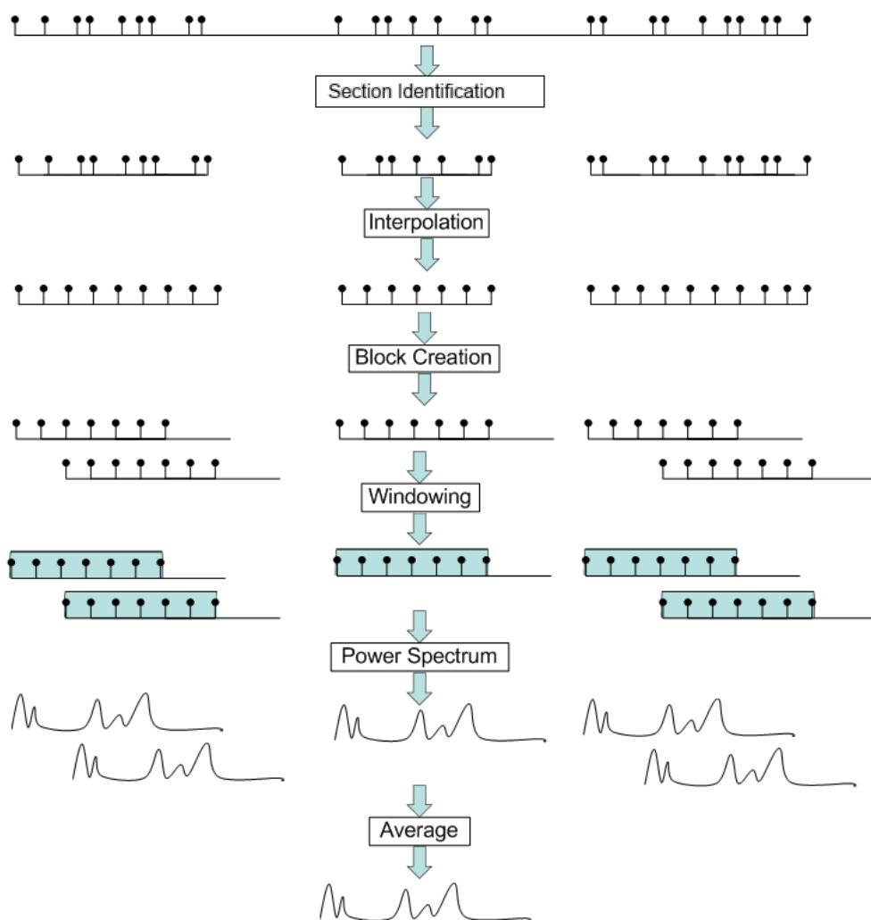
Figure 4-4: Calculating a parameter spectrum for non-contiguous pulses
