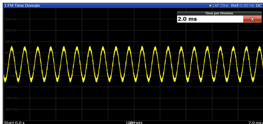
Figure 4-3: FM time domain measurement with time domain zoom (2.0 ms per division)
