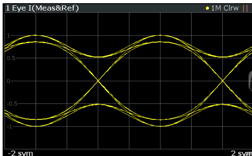
Figure 3-10: Eye Diagram Real (I) result display
