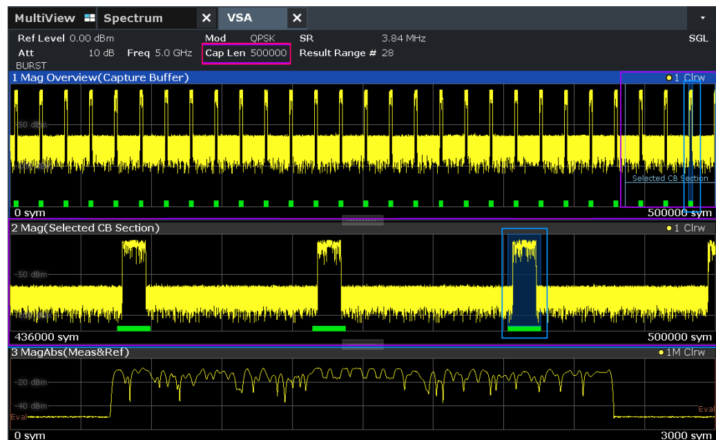
Figure 4-83: Magnitude absolute display for a long capture buffer
