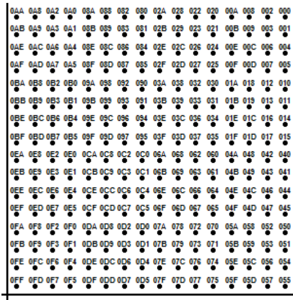
Figure 4-49: Constellation diagram for 1024QAM including the logical symbol mapping (hexadecimal); the figure shows the upper right section of the diagram only
