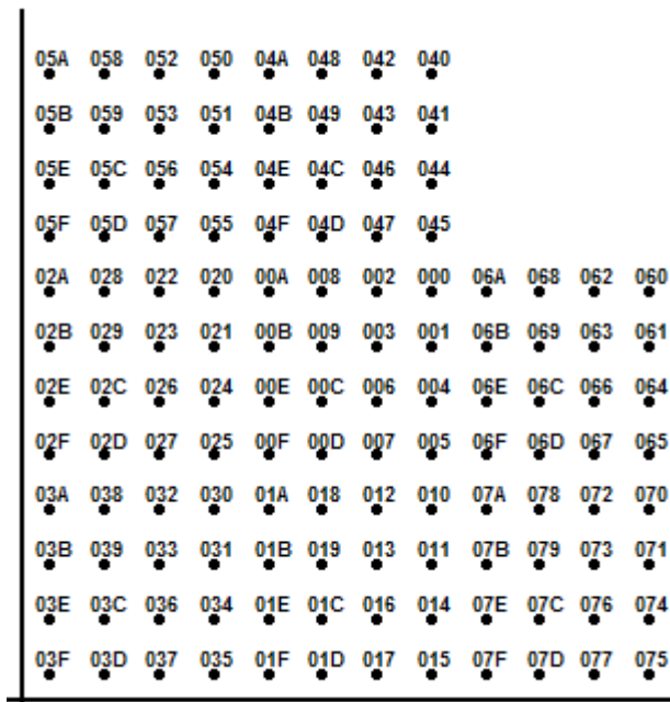
Figure 4-48: Constellation diagram for 512QAM (NATURAL, SMx), including the logical symbol mapping (hexadecimal); the figure shows the upper right section of the diagram only
