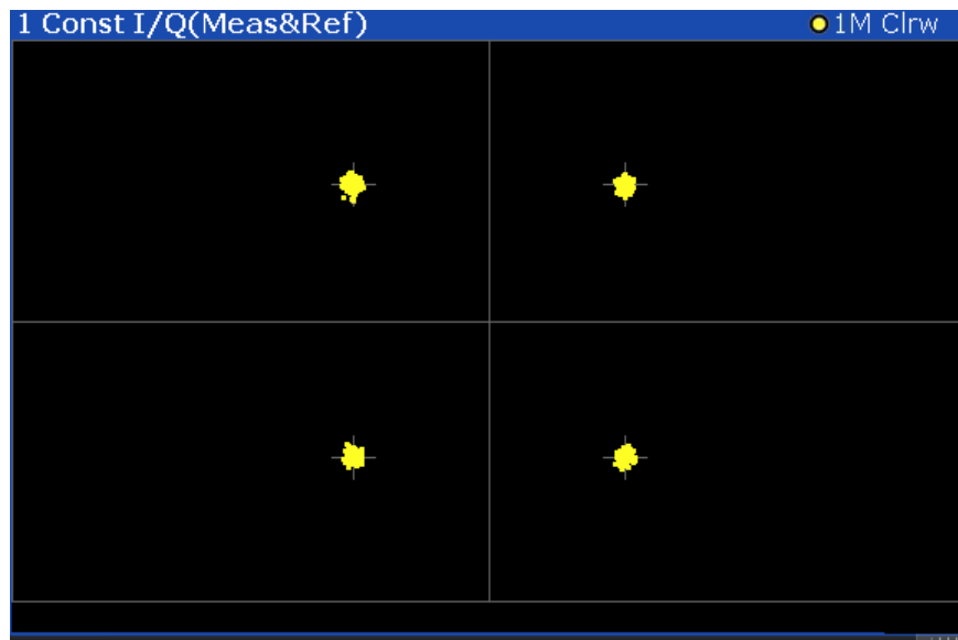
Figure 3-3: Constellation I/Q diagram for QPSK modulated signal
