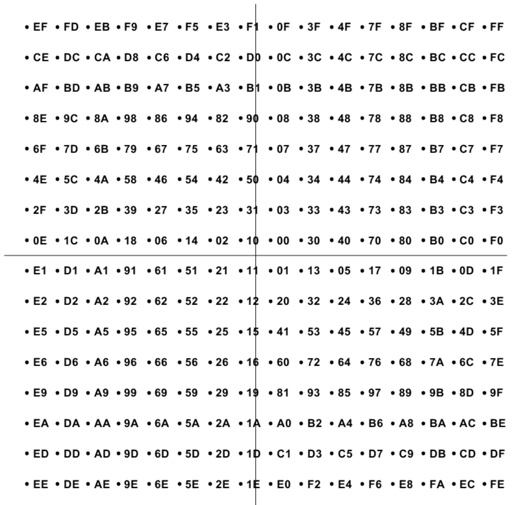
Figure 4-44: Constellation diagram for 64QAM including the logical symbol mapping for DOCSIS 3.0, North American Cable Downstream according to ITU-T J.83-B (hexadecimal)
