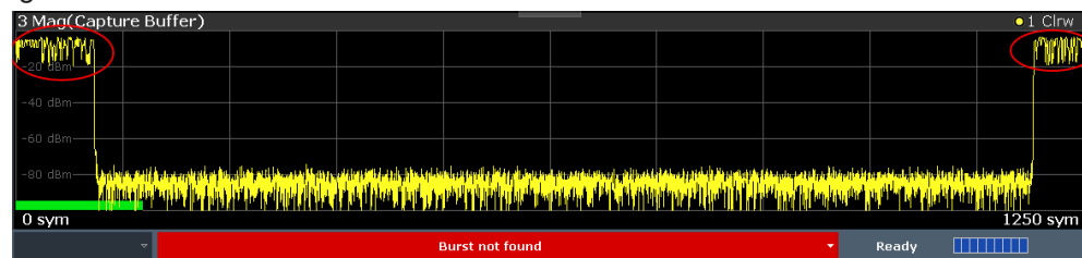
Figure 10-2: Example for incomplete burst capture
