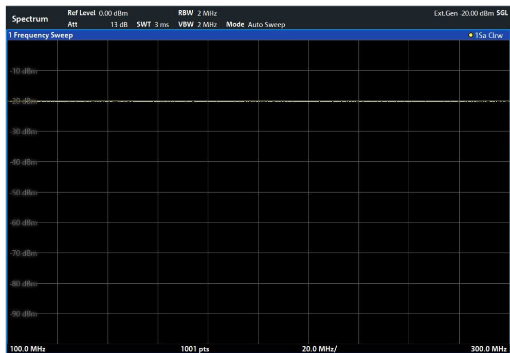
Figure 4-8: Measurement results from generator, analyzer and connecting cables
