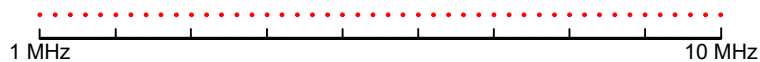
Figure 4-21: Linear x-axis scaling: the distance between the measurement points is equal, e.g. 200 kHz
