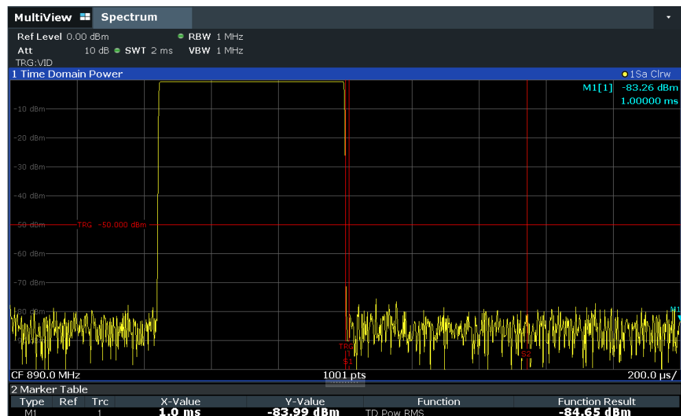
Figure 3-19: Measurement of the signal-to-noise ratio of a GSM burst signal in zero span
