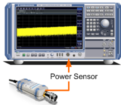
Figure 4-2: Connecting a power sensor using the POWER SENSOR interface
