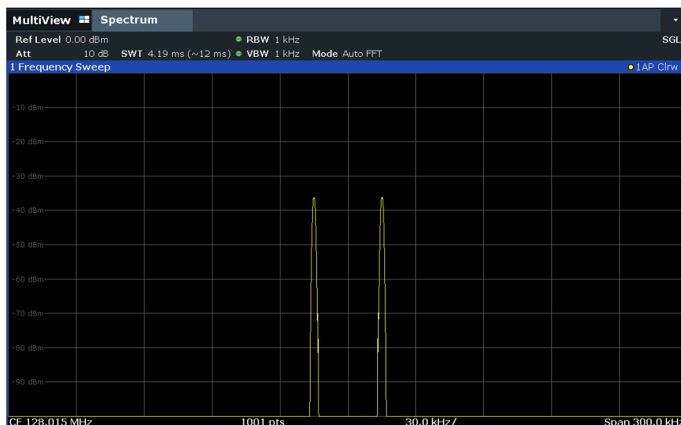
Figure 3-8: Measurement of two equally-leveled RF sinusoidal signals with a resolution bandwidth (1 kHz) which is significantly smaller than their frequency spacing
