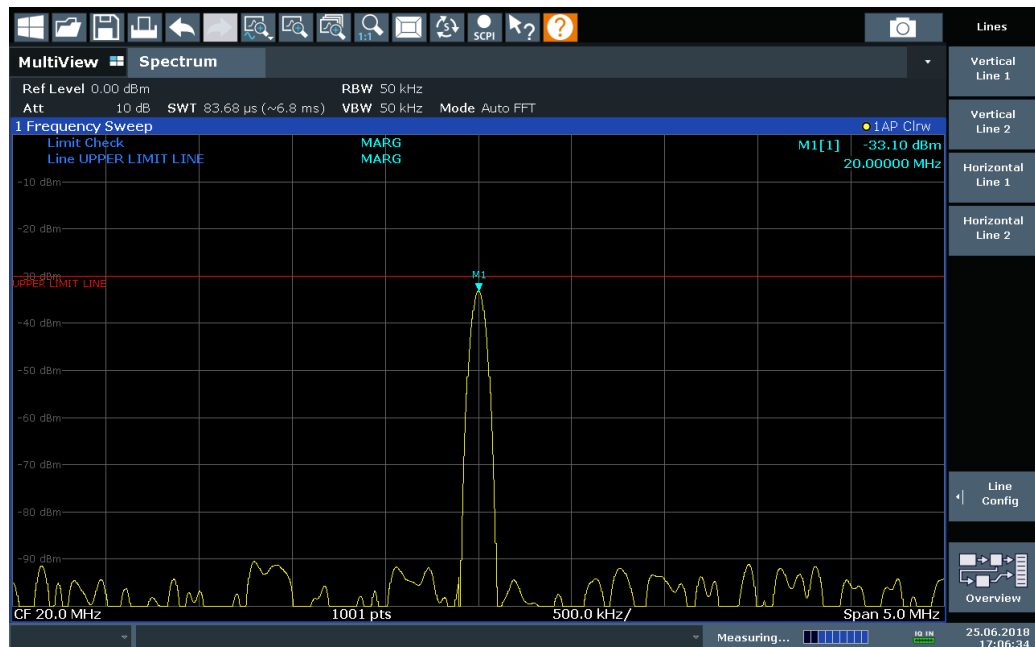
Figure 10-10: Margin violation for limit check
