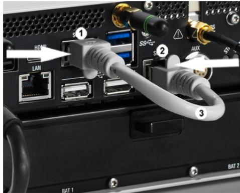
**Figure 6-2: Connection between scanner unit and internal PC unit**
