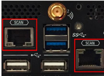
Figure 9-4: Connection ports for scanner link interconnection
