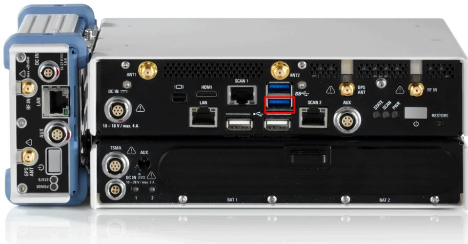
Figure 6-15: R&S TSMA with R&S TSMA-BP battery pack unit and mounted R&S TSME (rear side view, emphasized is USB 3.0 lower port)
