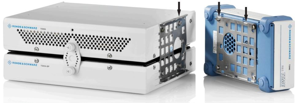
**Figure 6-17: Holders screwed on the devices**
