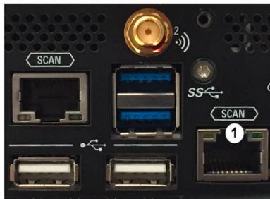
Figure 7-7: Scan ports of R&S TSMA
