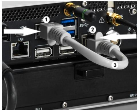
Figure 9-5: Connection between scanner unit and internal PC unit
