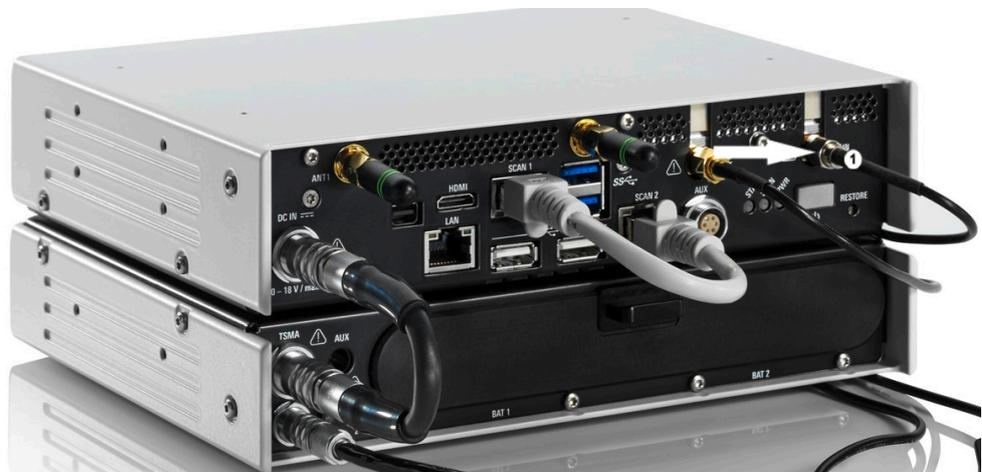
**Figure 9-8: R&S TSMA Antenna Cabling - RF**
