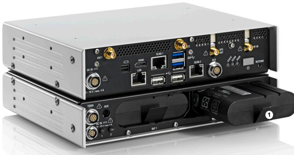
Figure 6-5: R&S TSMA - Battery Orientation
