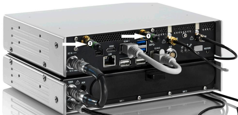
**Figure 9-9: R&S TSMA Antenna Cabling - WLAN and Bluetooth**
