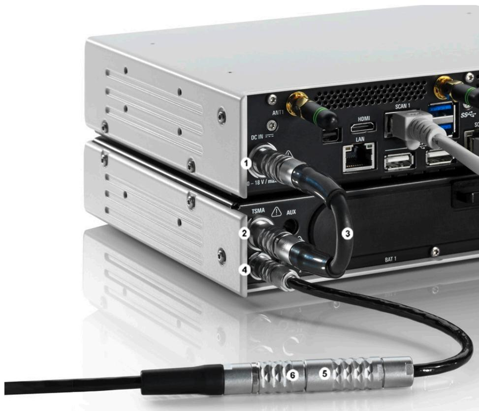
**Figure 6-13: Connecting the R&S TSMA with an AC power supply**
