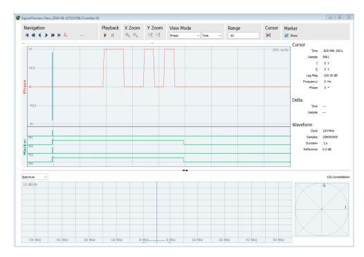
Figure 2-5: Signal Preview: Phase changes confirm the used Barker modulation (partial view, 10th pulse shown)
