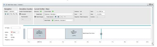
The "Mode Editor" is a graphical editor for joint configuration and defining the duration emitters are working in the different modes.
