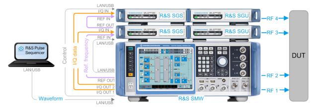
Figure 3-2: Direction finding setup for four individual RF channels up to 20 GHz
