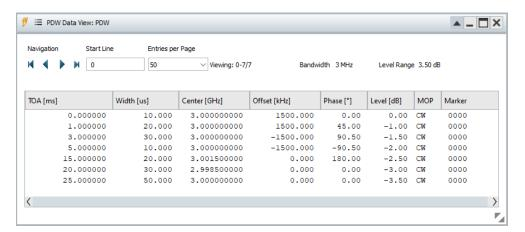
The dialog shows the waveform bandwidth, the level range and the waveform content as a sequence of pulses with their main characteristics.
