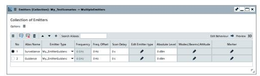
3. To observe and configure the properties of the individual emitters, select "Edit Emitter type". To configure attitude and behavior, select "Modes|Beams|Attitude".
