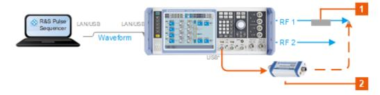
Figure 3-6: Path loss compensation (simplified setup)
