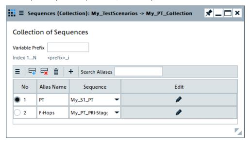
Switching between multiple sequences is possible in the pulse train sequential scenario.
