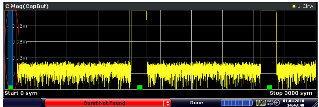
Figure 9-3: Example for measurement on incomplete burst capture
