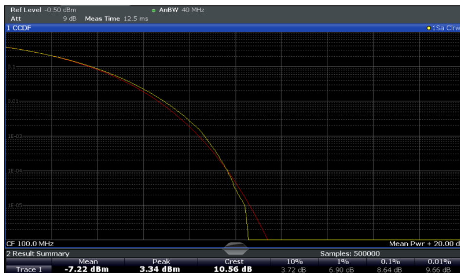
Figure 3-18: CCDF measurement results for the BTS application
