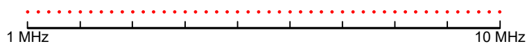
Figure 6-12: Linear x-axis scaling: the distance between the sweep points is equal, e.g. 200 kHz
