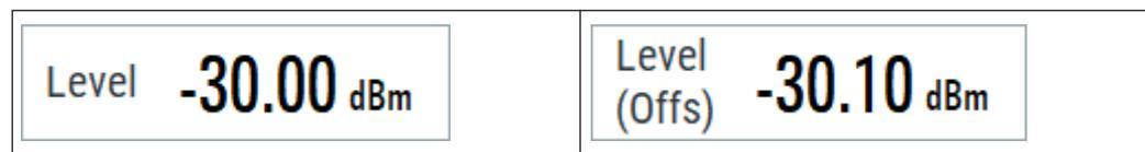
**Note:** The SCPI command `[ :SOURce ] :POWer [ :LEVel ] [ :IMMediate ] [ :AMPLitude ]` sets the level of the "Level" display, that means the level containing offset while `[ :SOURce ] :POWer :POWer` sets the level at the RF output connector.
