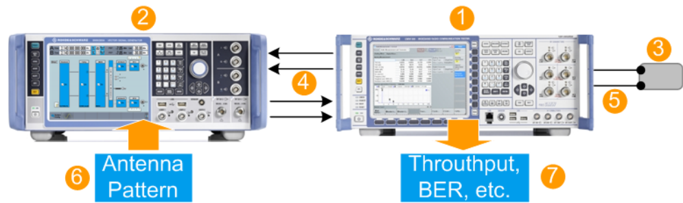
Figure 5-11: MIMO OTA testing: stage 2 (conducted setup)
