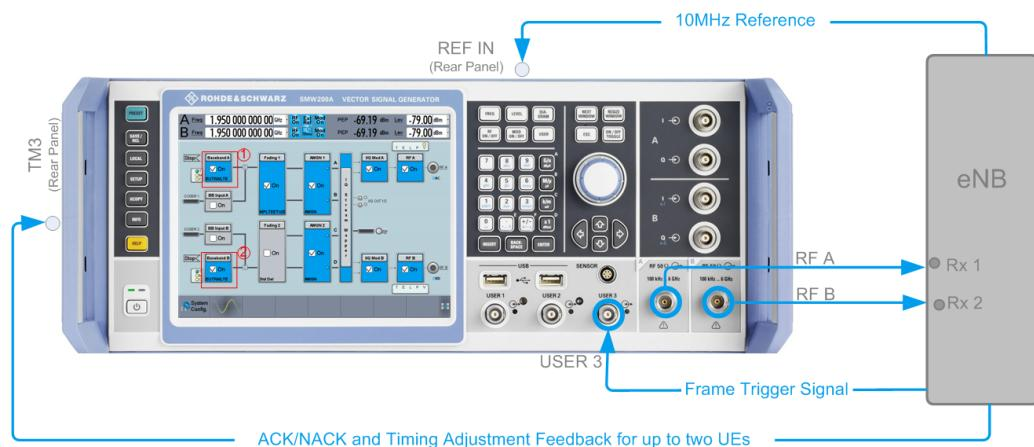
**Figure 5-2: Setup with R&S SMW-B10**
