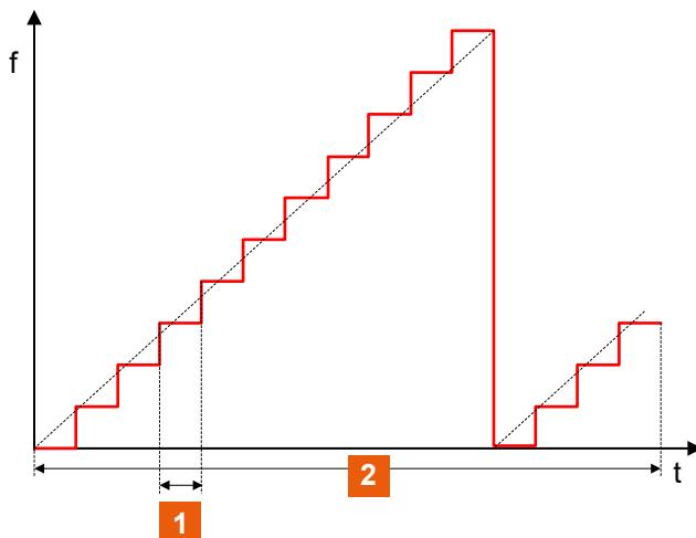
Figure 10-3: Sweep signal sawtooth shape
