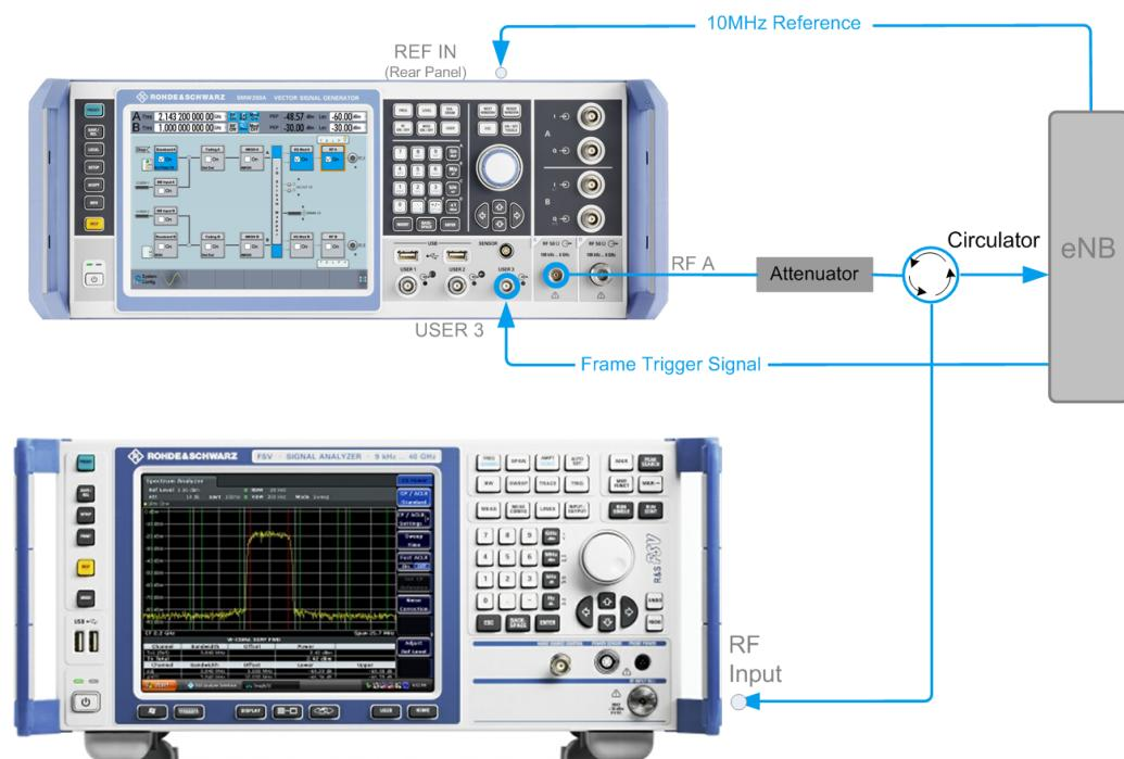
**Figure 8-6: Test setup for Test case 6.7: Transmitter Intermodulation**
