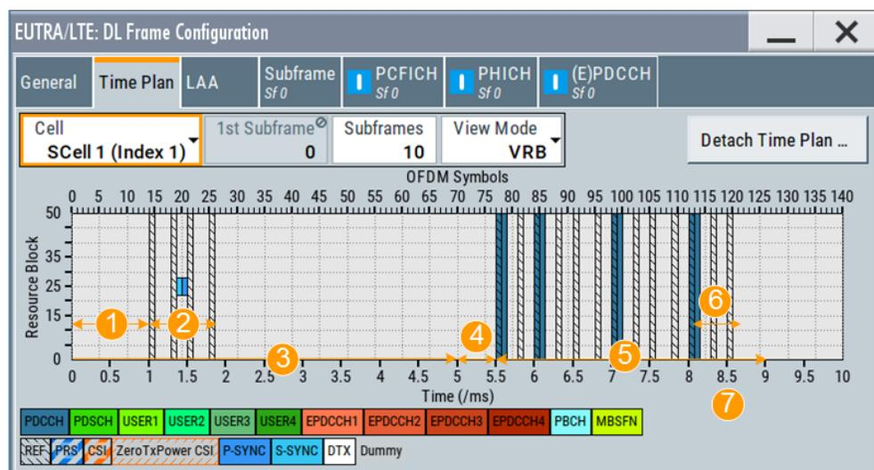
**Figure 4-12: LAA burst: understanding the displayed information**
