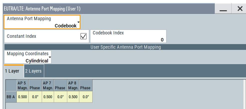
The available antenna ports and layers depend on the number of antennas and the transmission mode the UE is working in ("Frame Configuration > General > User > Tx Mode")
