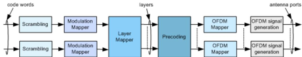
*Figure 2-25: Overview of downlink baseband signal generation*
