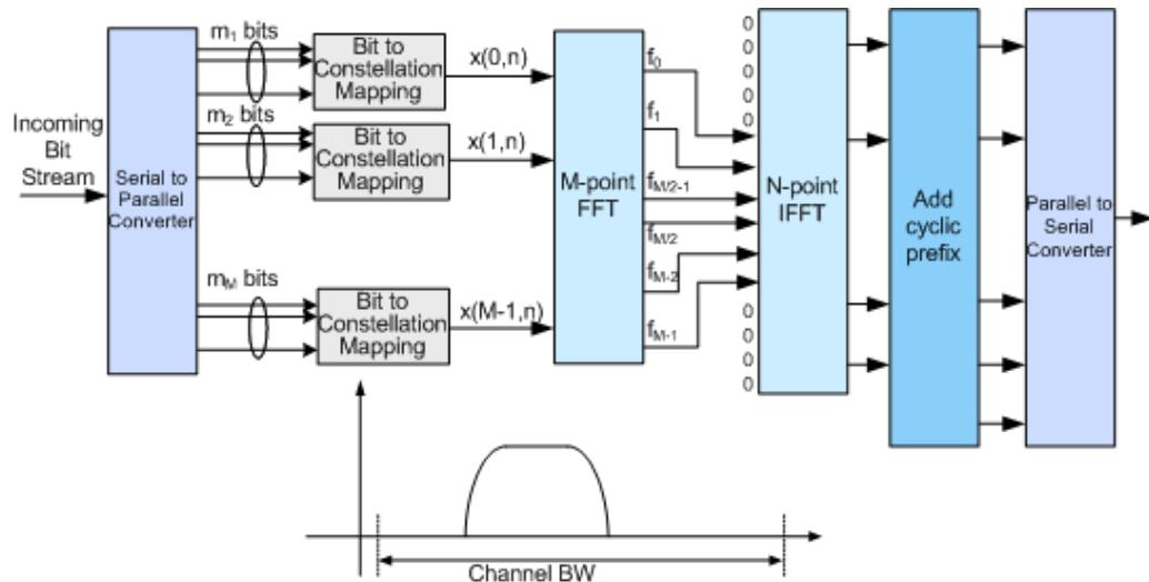
*Figure 2-16: Block diagram of DFT-s-OFDM (localized transmission)*
