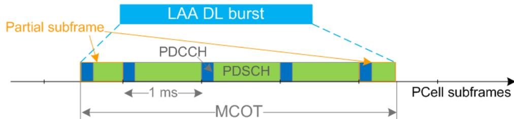
**Figure 2-34: DL LAA burst transmission**
