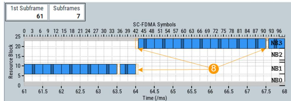
**Figure 6-8: Narrowband hop with PUSCH-to-PUSCH transition**
