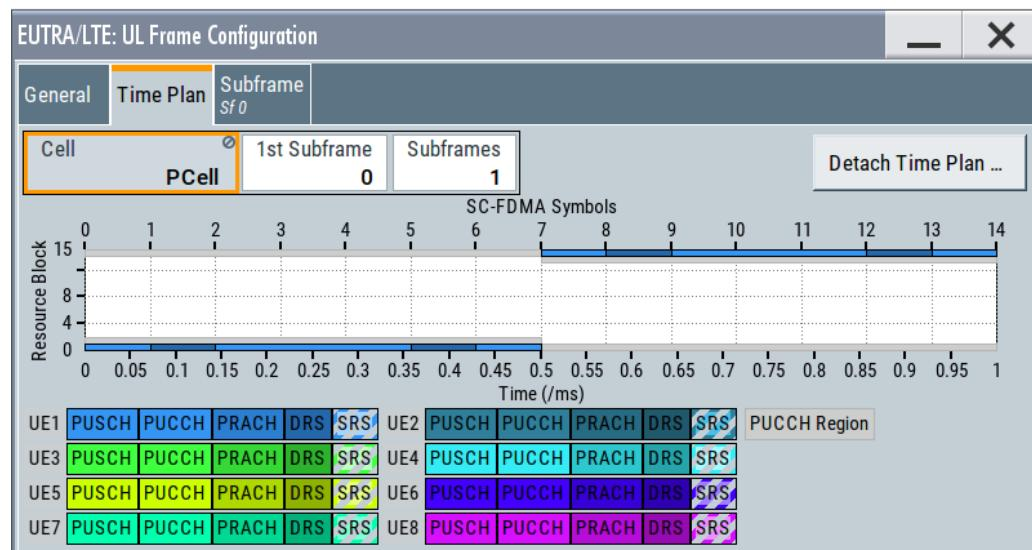
**Figure 4-15: Example: Representation of subframe with PUCCH region with three reserved resource blocks on the time plan**
