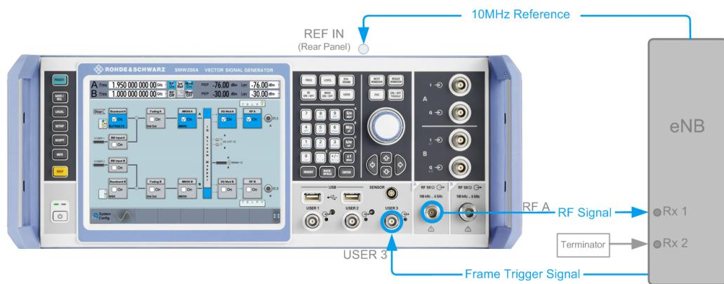
**Figure 8-1: One Path Standard Test Setup (Example of R&S SMW simulating the test case 7.3 "Dynamic Range")**
