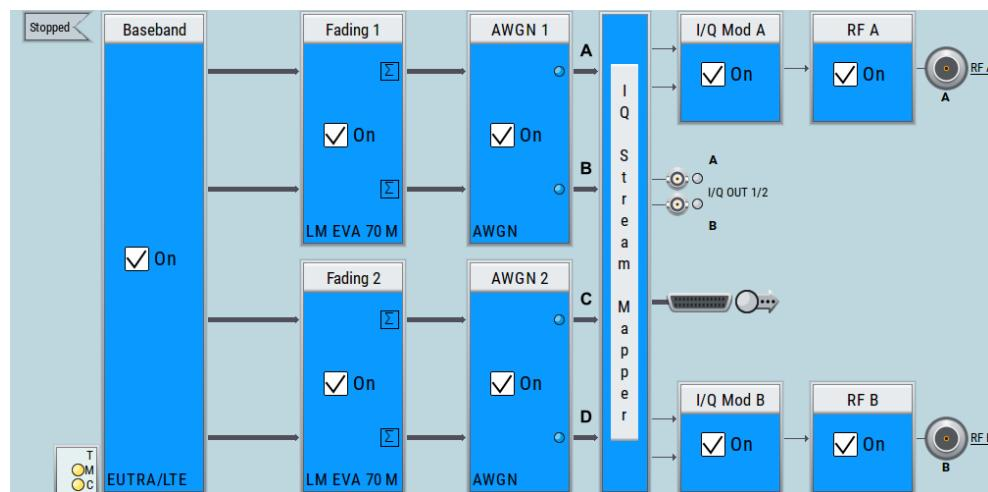
Figure 4-2: Example: Intra-band 2x2x2 LTE carrier aggregation
