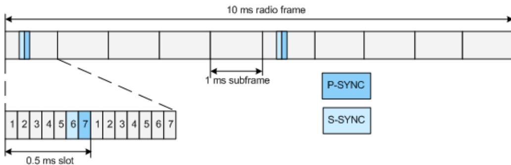
*Figure 2-10: P-SYNC and S-SYNC structure (normal CP; 1.25 MHz bandwidth)*
