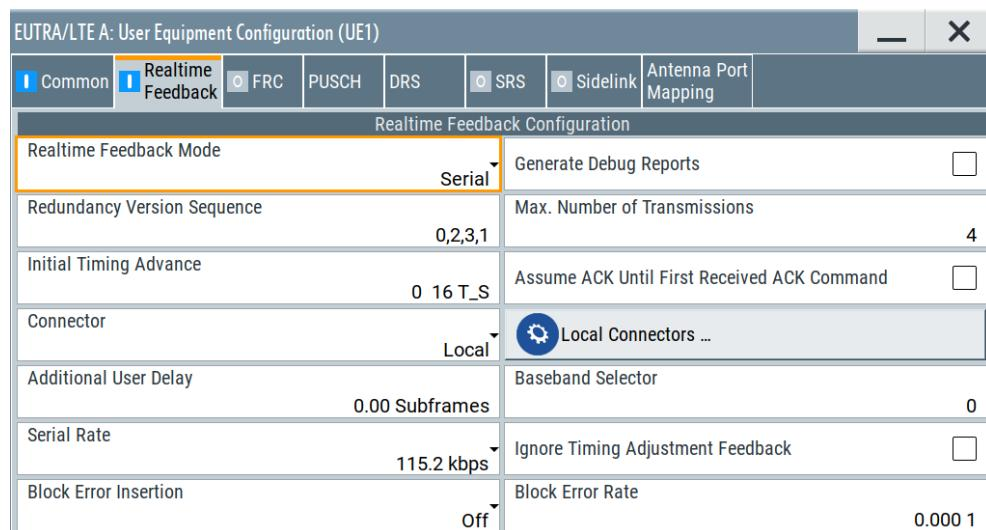
This dialog provides access to the parameters required for generating signals in accordance to the HARQ feedback or UL timing adjustments test cases. The provided parameters depend on the selected **Realtime Feedback Mode**.
