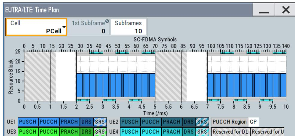
Figure 7-2: TDD time plan (UL)
