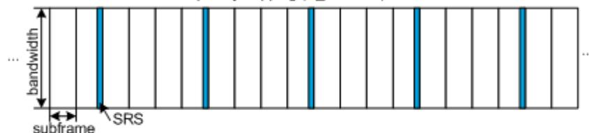
SRS transmission with frequency hopping ( $B_{SRS} \neq 0$ )
