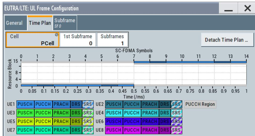
**Figure 6-21: Example: Representation of subframe with PUCCH region with three reserved resource blocks on the time plan**
