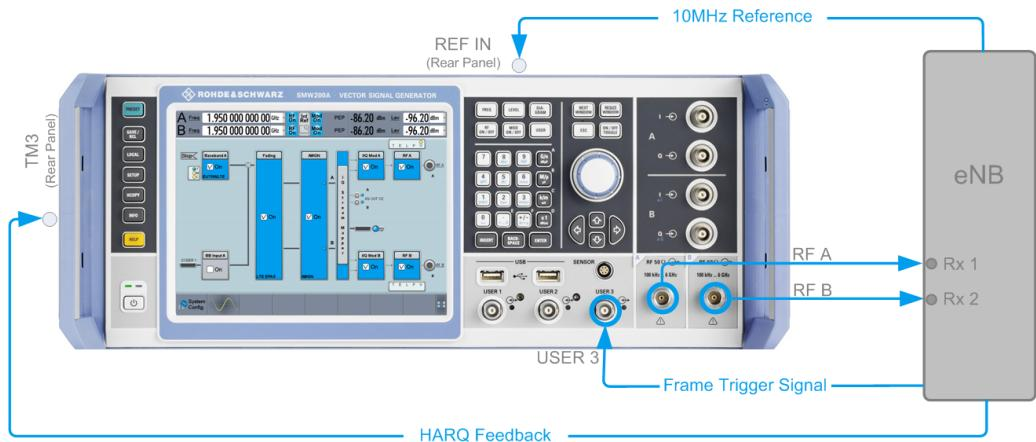
**Figure 8-3: Test Setup for Diversity Measurements (Example of R&S SMW simulating test case 8.2.1 "PUSCH in Multipath Fading Propagation Conditions" with two Rx antennas)**
