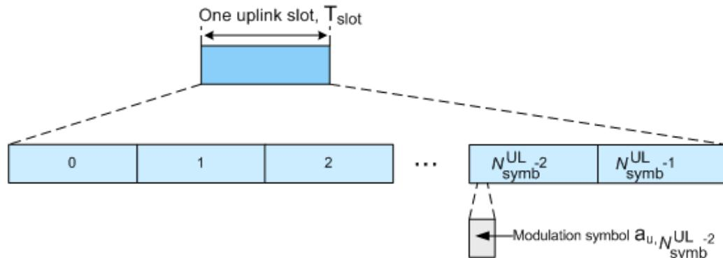
*Figure 2-17: Uplink slot structure*
