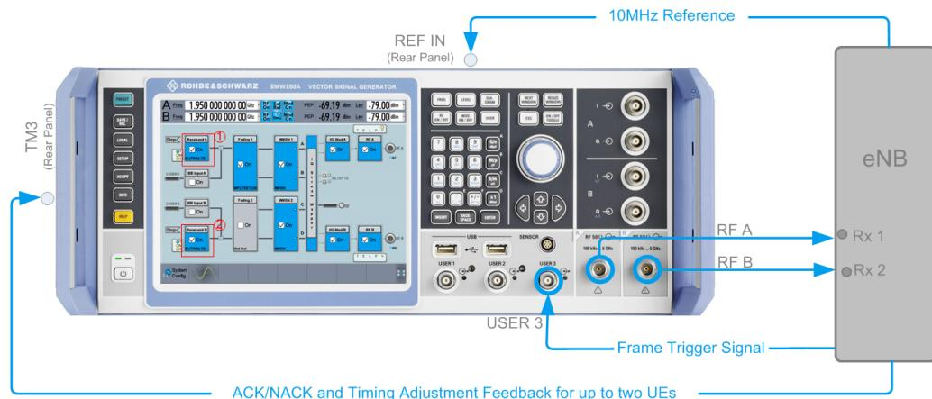
**Figure 8-13: Test Setup for test case 8.2.2 "UL Timing Adjustment"**
