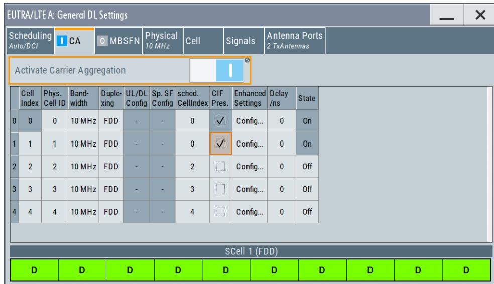
Figure 4-1: General DL Settings > Carrier Aggregation dialog in System Config > Fading and Baseband Configuration > BB Source Config > Coupled Sources
