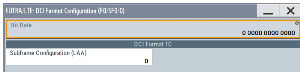
If LAA is used, the DCI format 1C carries information about the LAA subframe configuration.
