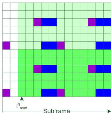
**Figure 6-14: NPDCH mapping [1MA266]**
