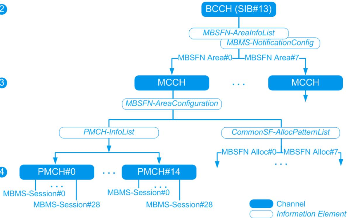
Figure 4-5: MBSFN Signaling (steps 2 to 4)
