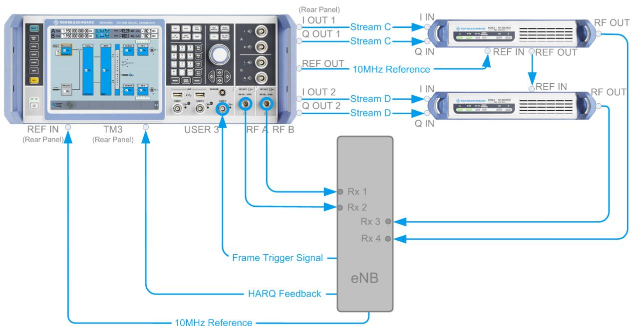
**Figure 8-4: Test Setup for tests with four Rx antennas (Example of R&S SMW and 2xR&S SGS simulating test case 8.2.1 "PUSCH in Multipath Fading Propagation Conditions")**
