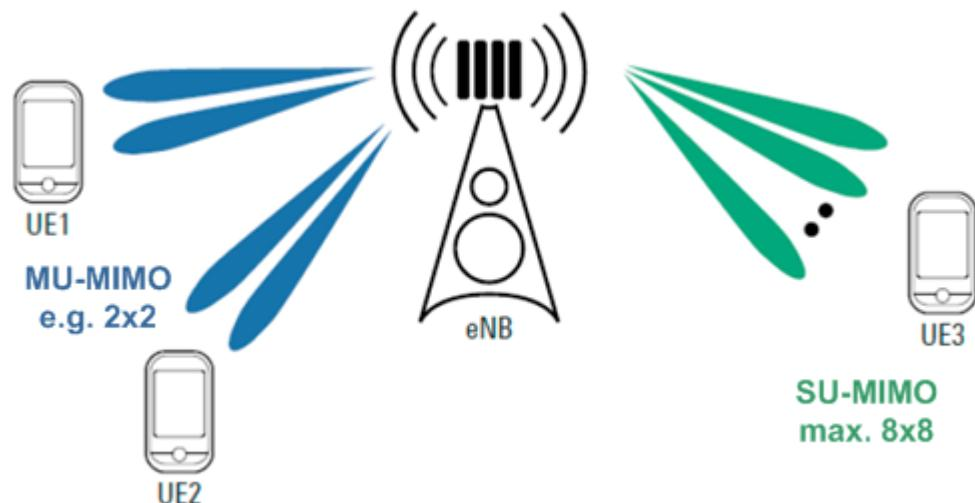
*Figure 2-29: Supported transmit layers in LTE-Advanced (downlink)*
