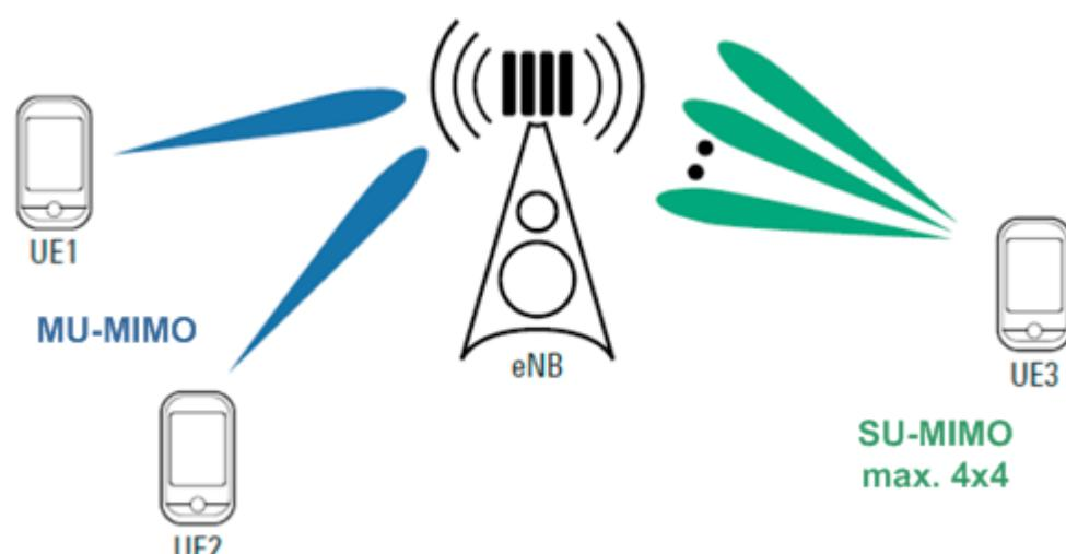
*Figure 2-30: Supported transmit layers in LTE-Advanced (uplink)*
