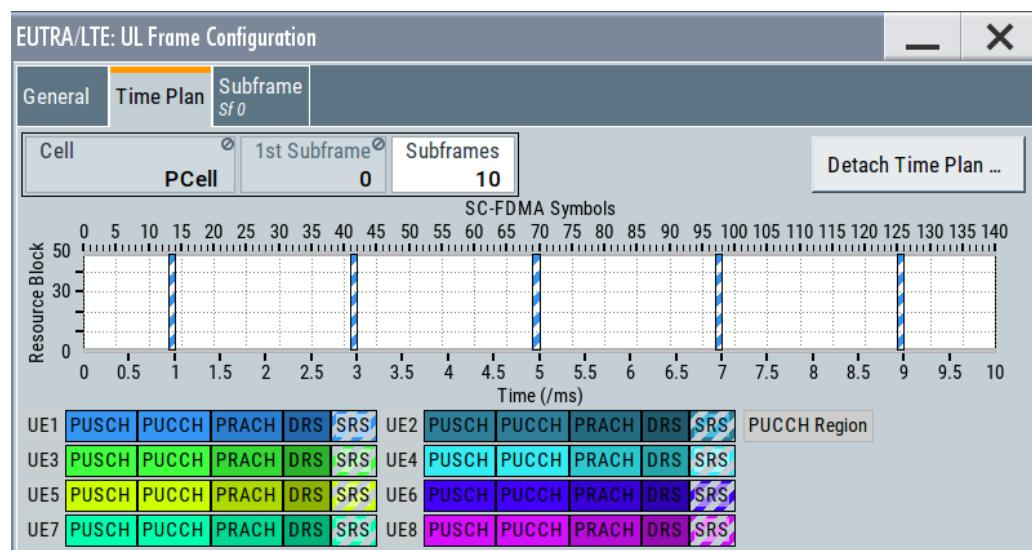
Changing the SRS bandwidth to " $B_{SRS} = 3$ " results in the most narrowband SRS transmission with SRS bandwidth of 4 RBs and enabled frequency hopping.
