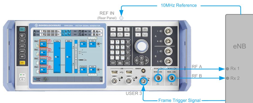
**Figure 8-14: Test Setup for test case 8.3.3 "ACK missed detection for multi-user PUCCH format 1a"**
