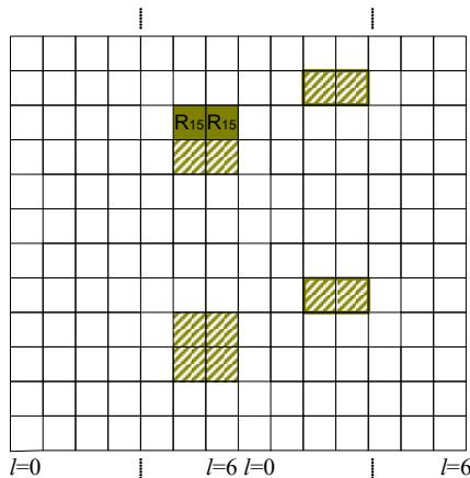
*Figure 2-15: Mapping of a CSI-RS on antenna port 15 (CSI configuration 0, normal cyclic prefix)*
