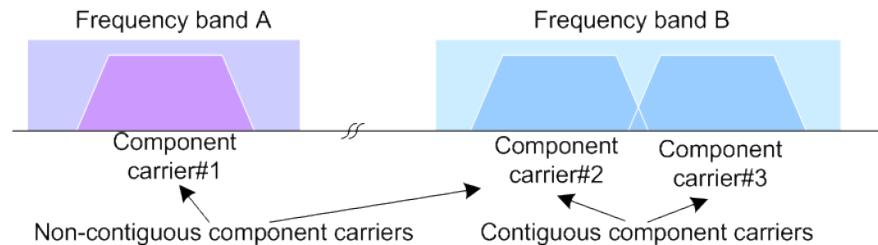
**Figure 2-26: Carrier aggregation**
