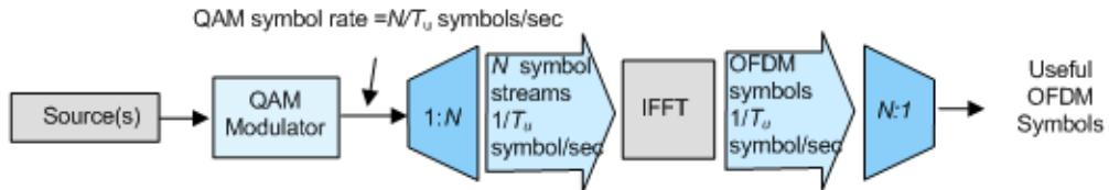
**Figure 2-2: OFDM signal generation chain (3GPP TR 25.892)**
