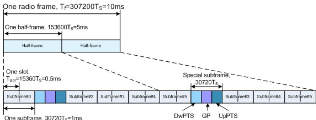
**Figure 2-4: Frame format 2 (TDD mode), 5 ms switching periodicity**
