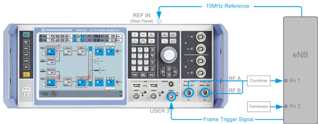
**Figure 8-2: Two Paths Standard Test Setup (Example of R&S SMW simulating test case 7.8 "Receiver Intermodulation")**
