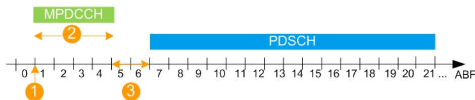
*Figure 6-4: Example of MPDCCH repetitions and PDSCH cross-scheduling (UE-specific search space)*
