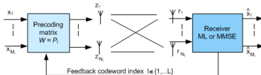
*Figure 2-24: Precoding principle*
