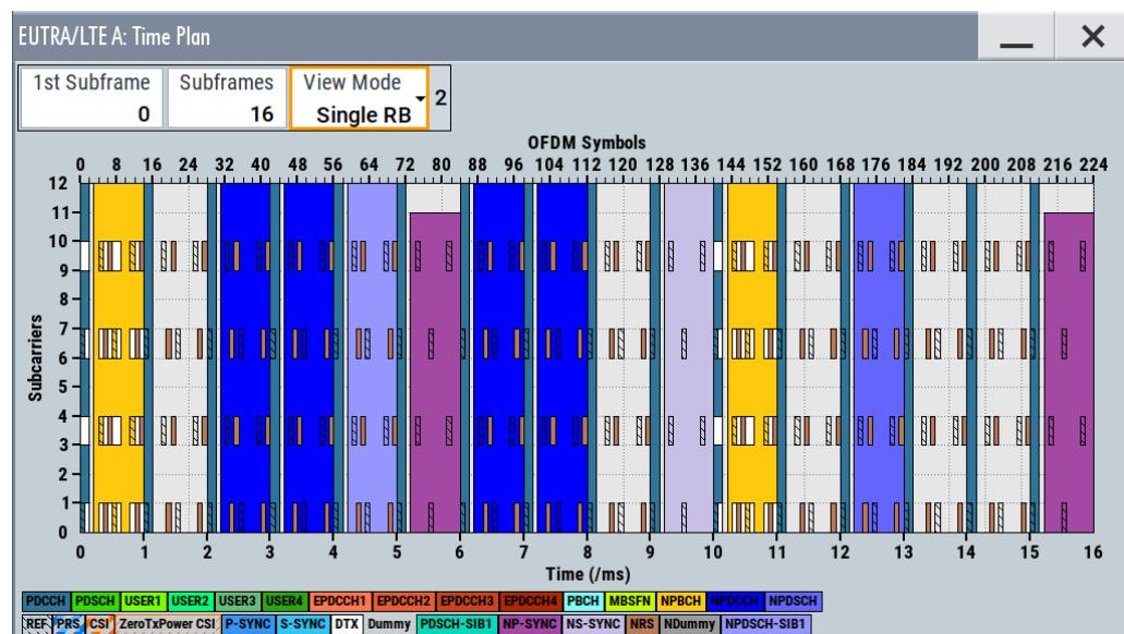
[Figure 6-15: NPDCH scheduling based on DCI format N1](#)
