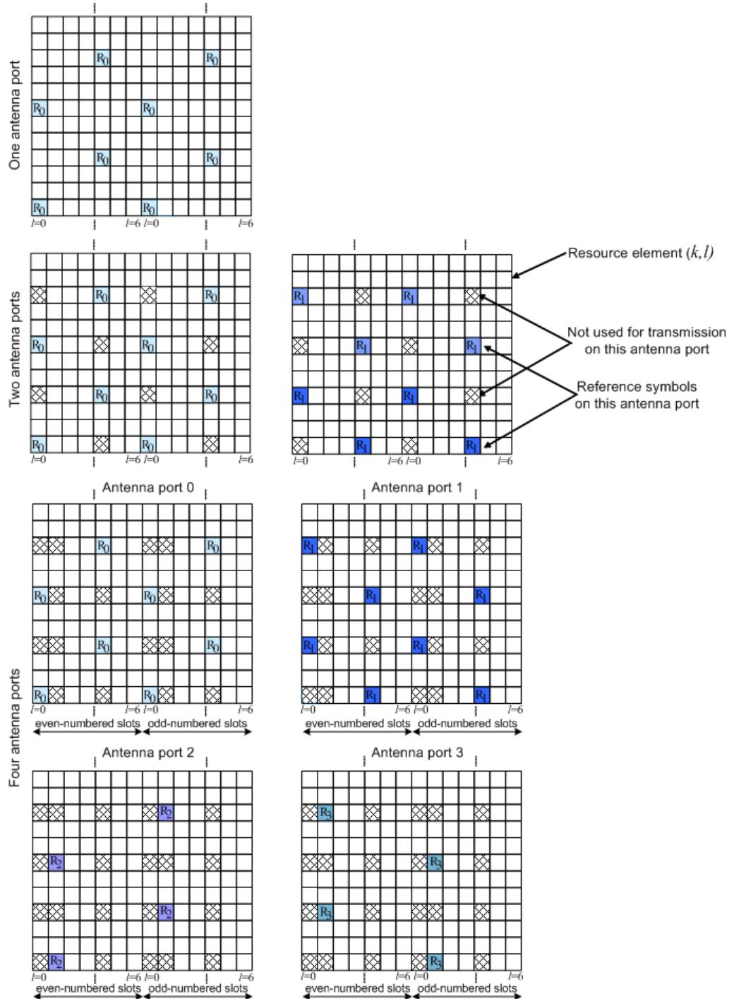
Figure 2-9: Downlink reference signal structure (normal cyclic prefix)
