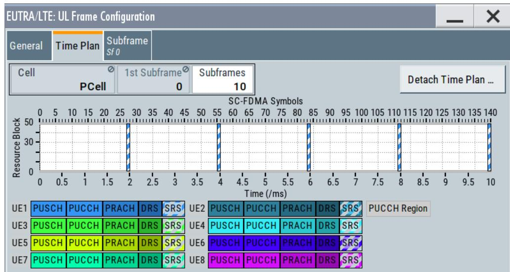
For TDD duplexing mode, a  $T_{offset}$  of 0 or 5 means that SRS is transmitted in the second last symbol of the special subframe (in the UpPTS part). For this case, adjust the parameter [TDD Special Subframe Config](#) so that an UpPTS field length of two symbols is assured.
