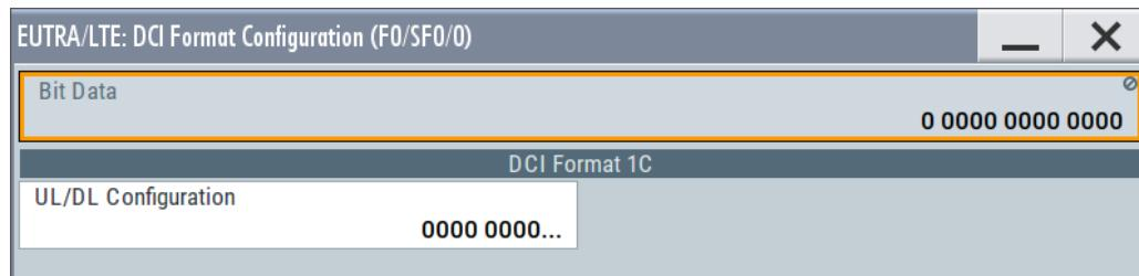
If eIMTA is used, the DCI format 1C carries information about the UL/DL configuration numbers. Each UL/DL configuration number consists of 3 bits and indicates one of the configurations listed in [Figure 2-5](#).
