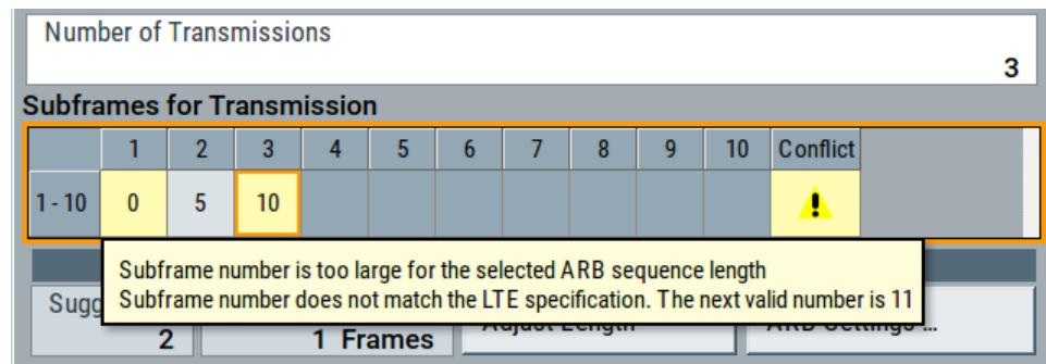
**Figure 4-16: Example of conflict indication: DCI 4 Set 2 and DCI 1A/2B/2C/2D SRS sets use configuration index (subframe number) = 2**
