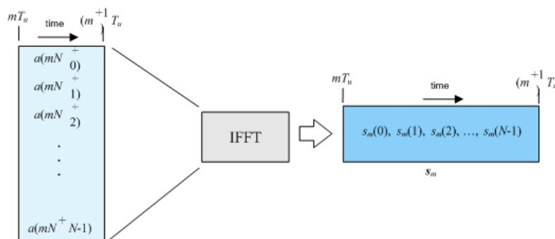
**Figure 2-1: OFDM useful symbol generation using an IFFT (3GPP TR 25.892)**
