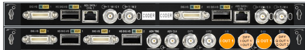
Figure 4-4: Wideband baseband instrument rear panel: Analog output interfaces
