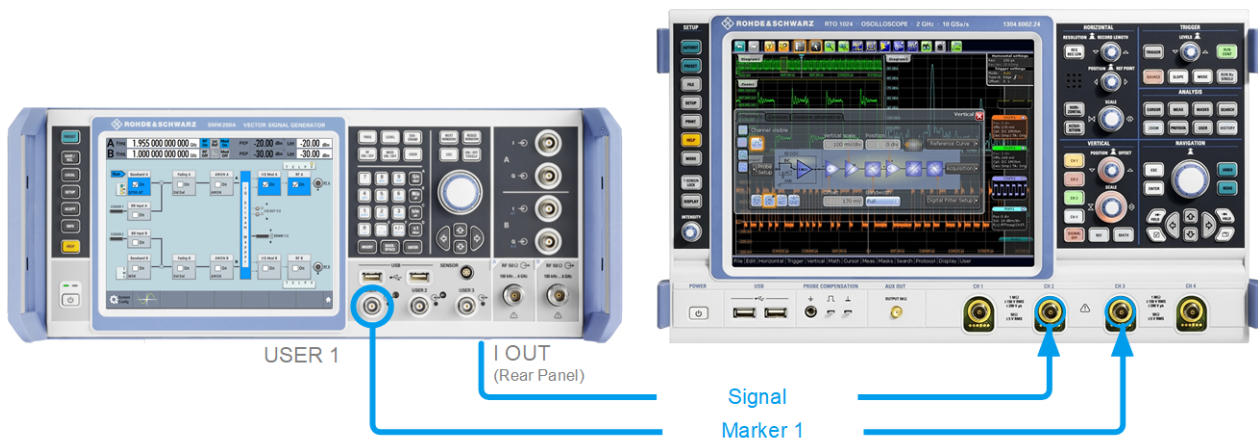
Figure 3-15: Simplified representation of a test setup for signal monitoring**
