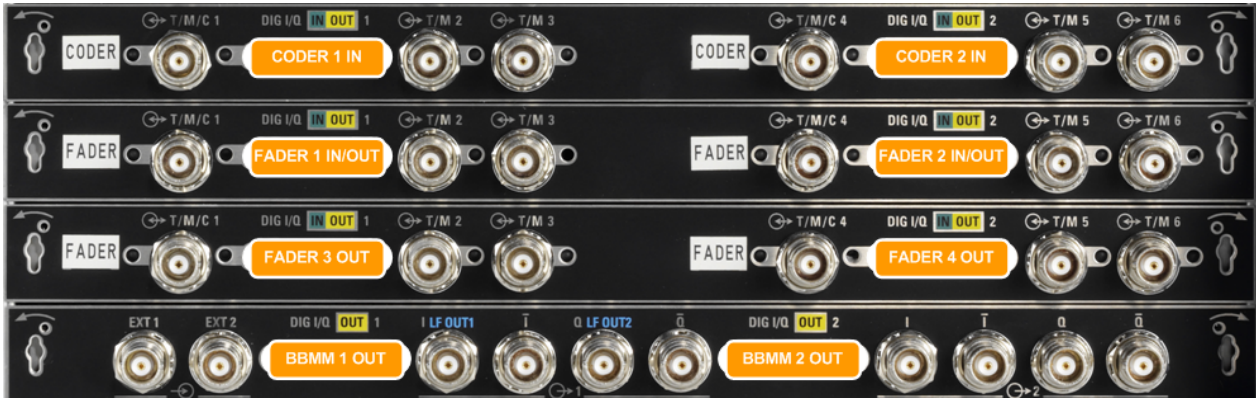
Figure 4-1: Location of the digital input and output interfaces (part view of the rear panel of a fully equipped instrument, standard baseband)
