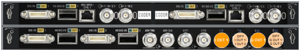
Figure 4-4: Location of the analog output interfaces (part view of the rear panel of a fully equipped instrument, wideband baseband)
