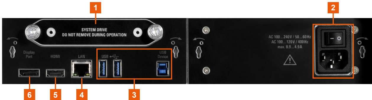
Figure 3-6: Processing board connectors and power supply
