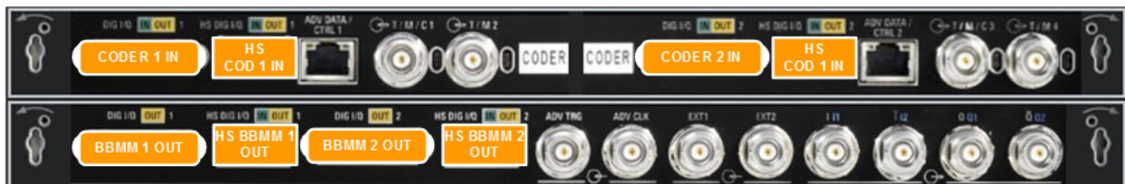
Figure 4-2: Location of the digital input and output interfaces (part view of the rear panel, wide-band baseband)
