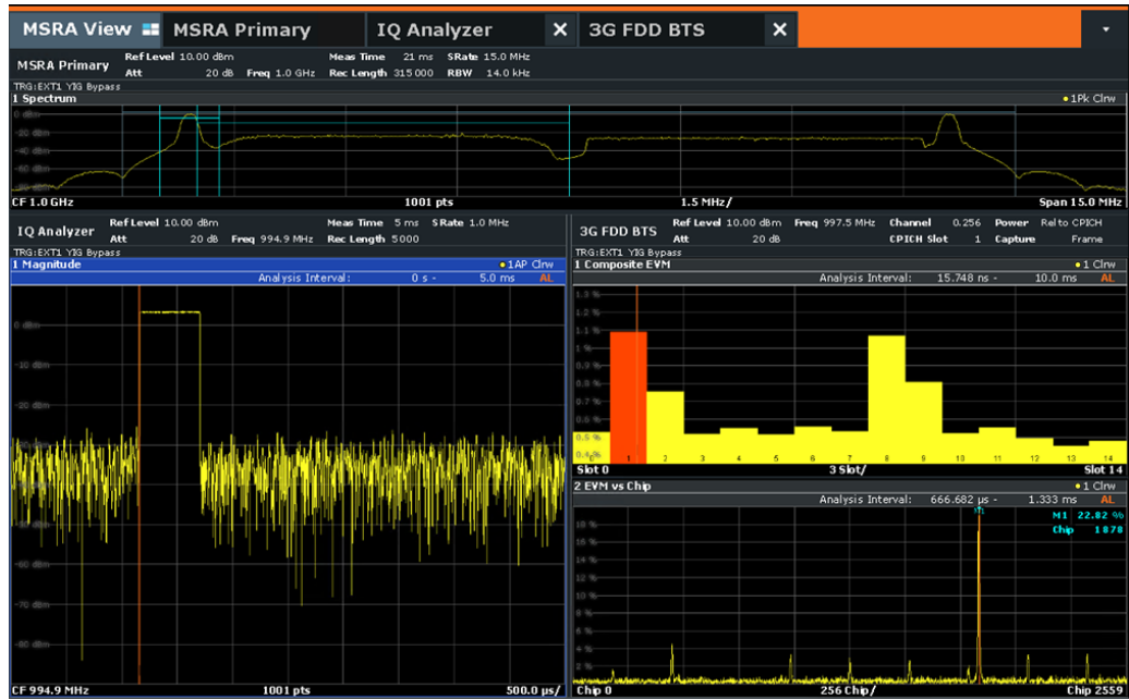
Figure 10-5: MSRA View of MSR signal with time correlations
