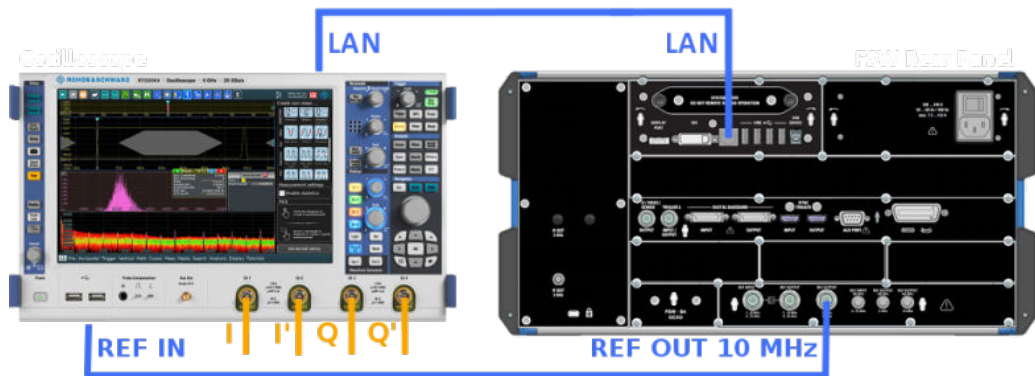
Figure 5-20: Measurement setup with the optional Oscilloscope Baseband Input
