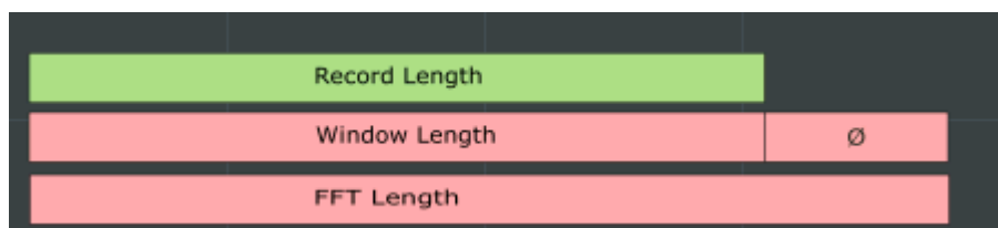
Figure 5-28: FFT parameters for single FFT calculation
