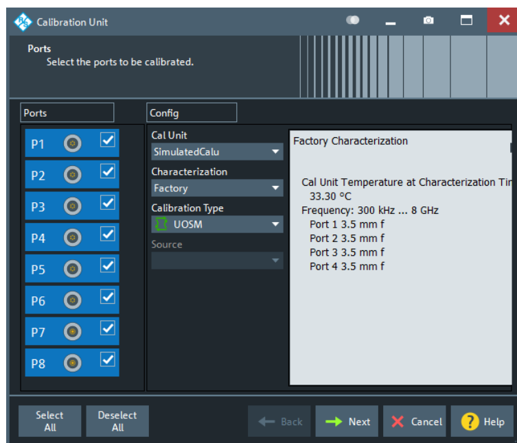
Figure 5-12: Calibration Unit wizard, step 1: Ports (> 4 test ports)
