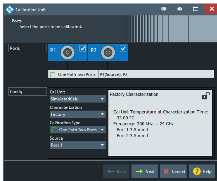
Figure 5-10: Calibration Unit wizard, step 1: Ports
