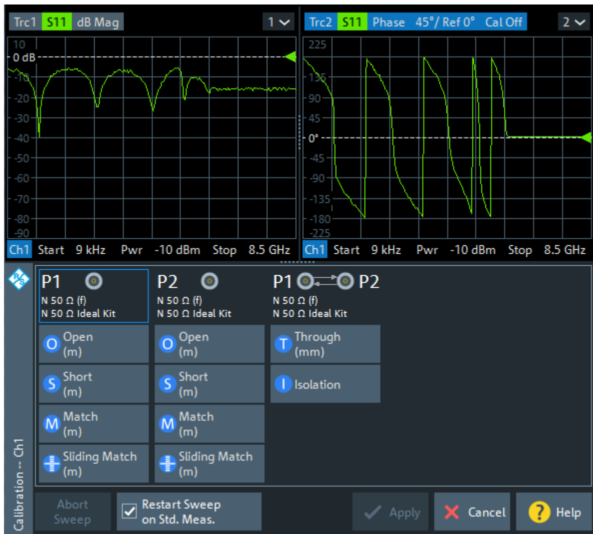
Figure 5-18: Calibration Setting Wizard, Step 3: Calibration
