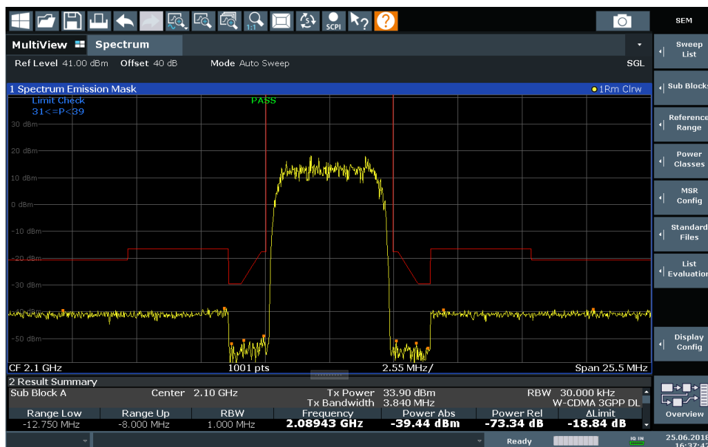
Figure 6-45: Detected peak display in SEM measurement
