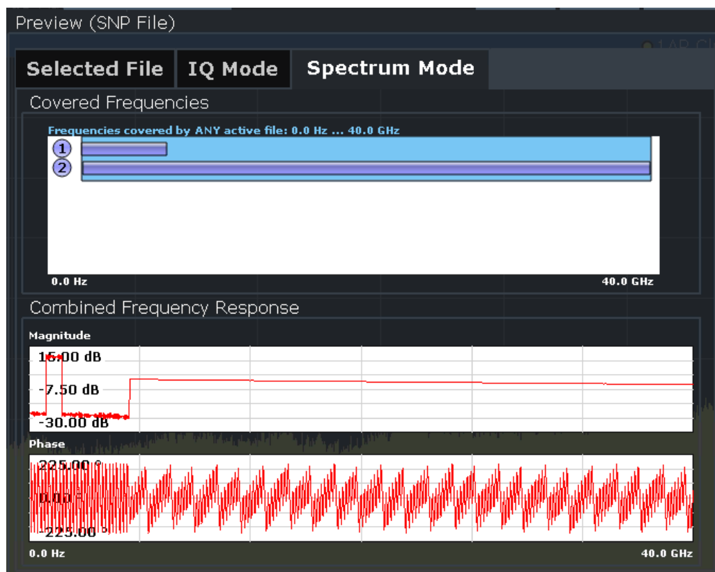
Figure 11-3: Spectrum Mode preview of user correction files
