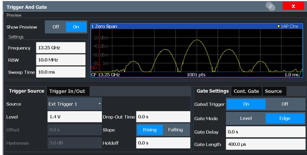
External triggers from one of the TRIGGER INPUT / OUTPUT connectors on the FSW are configured in a separate tab of the dialog box.
