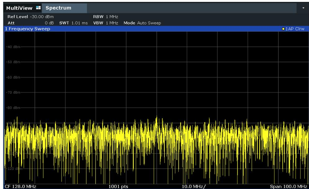
Figure 6-1: Sine wave signal with low S/N ratio
