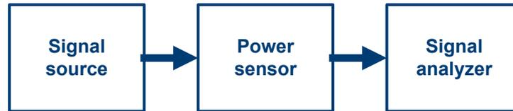
Figure 7-12: Power sensor support – standard test setup
