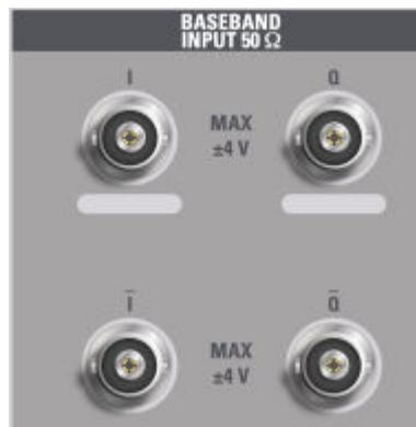
The upper BNC connectors BASEBAND INPUT I and BASEBAND INPUT Q are used to input:
