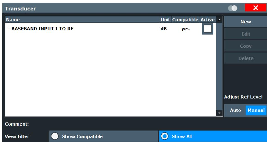
For the transducer line overview, the FSW searches for all stored transducer lines with the file extension .TDF in the C:\Program Files (x86)\Rohde-Schwarz\FSW\\trd directory. The overview allows you to determine which transducer lines are available and can be used for the current measurement.
