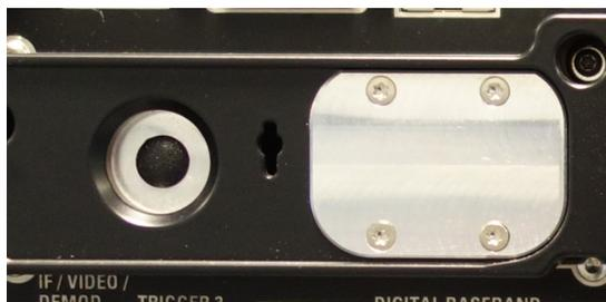
The output connector provides I/Q data streams with a sample rate of up to 600 MHz, if the R&S FSW-B517 option is installed and active. With R&S FSW-B1017 installed, output rates up to 1200 MHz are available.
