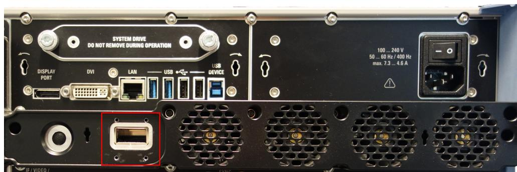
If necessary, remove the metal cover from the connector on the rear panel of the FSW.
