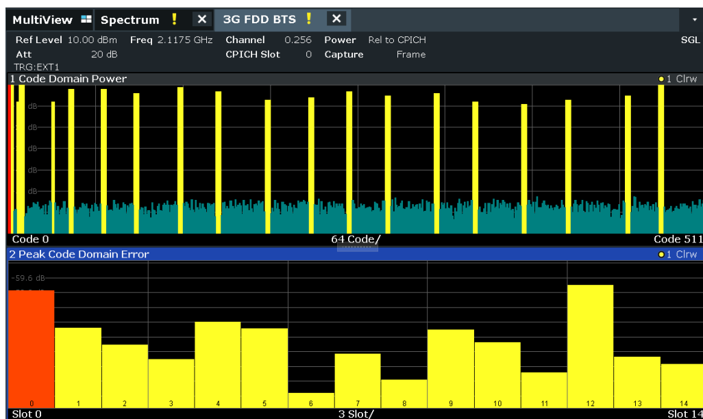
Figure 10-8: Measurement Example 6: Determining the Peak Code Domain Error
