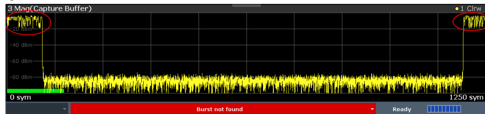
Figure 10-2: Example for incomplete burst capture
