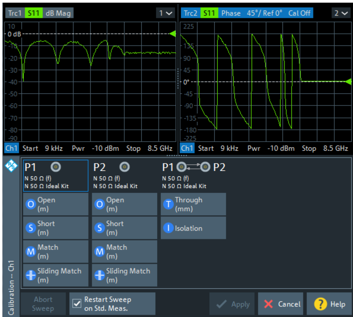
Figure 5-27: Calibration Setting Wizard, Step 3: Calibration
