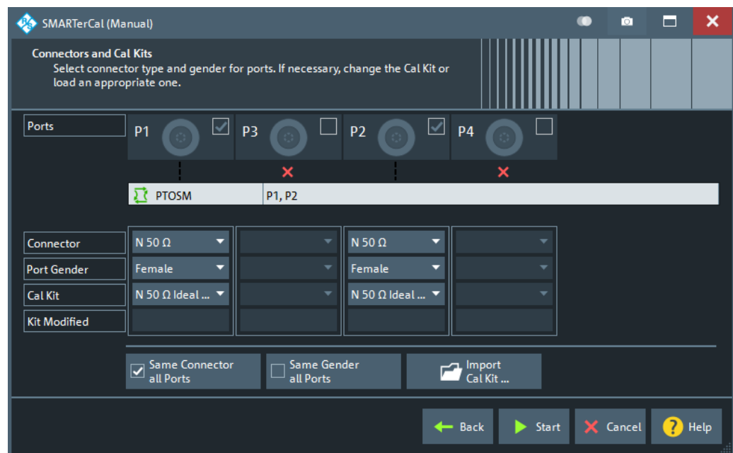
Figure 5-42: SMARTerCal(Manual), Step 2: Connectors and Cal Kits
