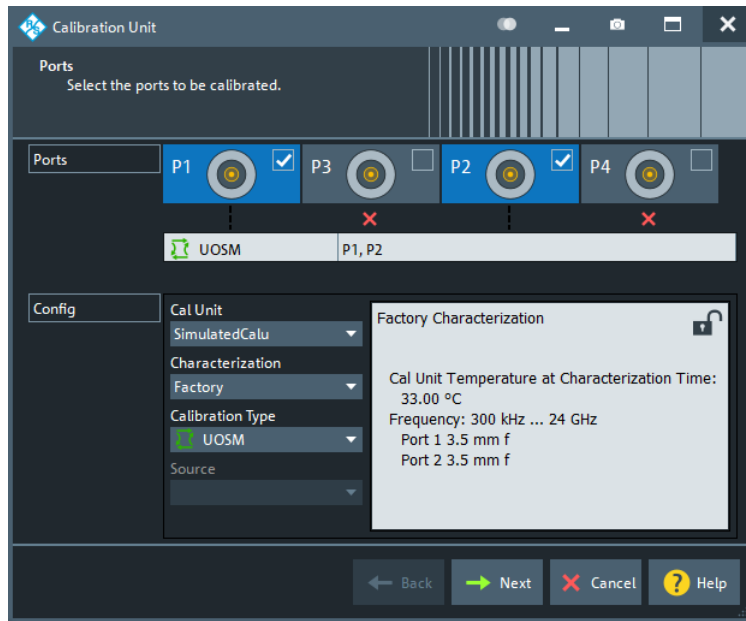
Figure 5-12: Calibration Unit wizard, step 1: Ports
