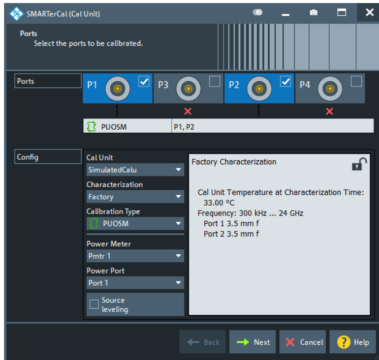
Figure 5-30: SMARTerCal (Cal Unit), Step 1: Ports
