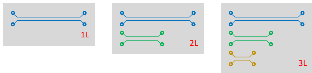
Figure 4-26: Test coupons for 1L, 2L and 3L measurements
