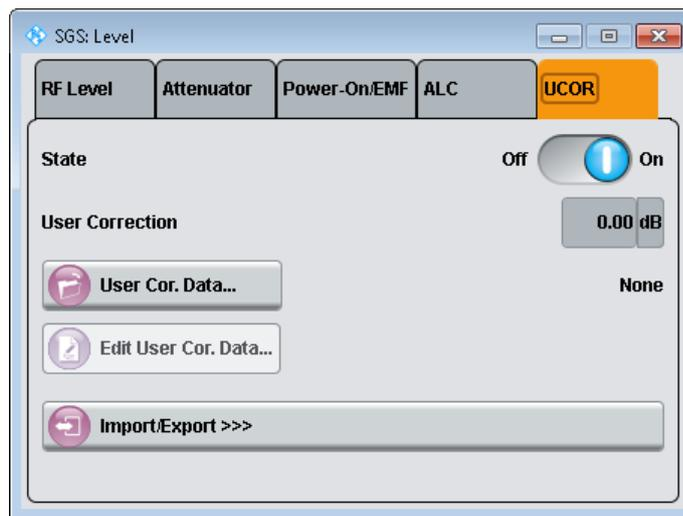
The "User Correction" function is used to create and activate lists in which level correction values predefined by the user are freely assigned to RF frequencies. Correction is performed by the user-defined table values being added to the output level for the respective RF frequency.
