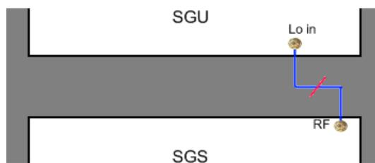
**Figure 9-10:** A faulty connection between an R&S SGU and an R&S SGS
