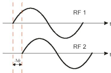
If two signal generators are coupled via their 10 MHz reference, they are generating the same frequency but only in the long-term perspective. The instantaneous differential phase (“delta phase”) of these two RF signals is unstable due to the following:
