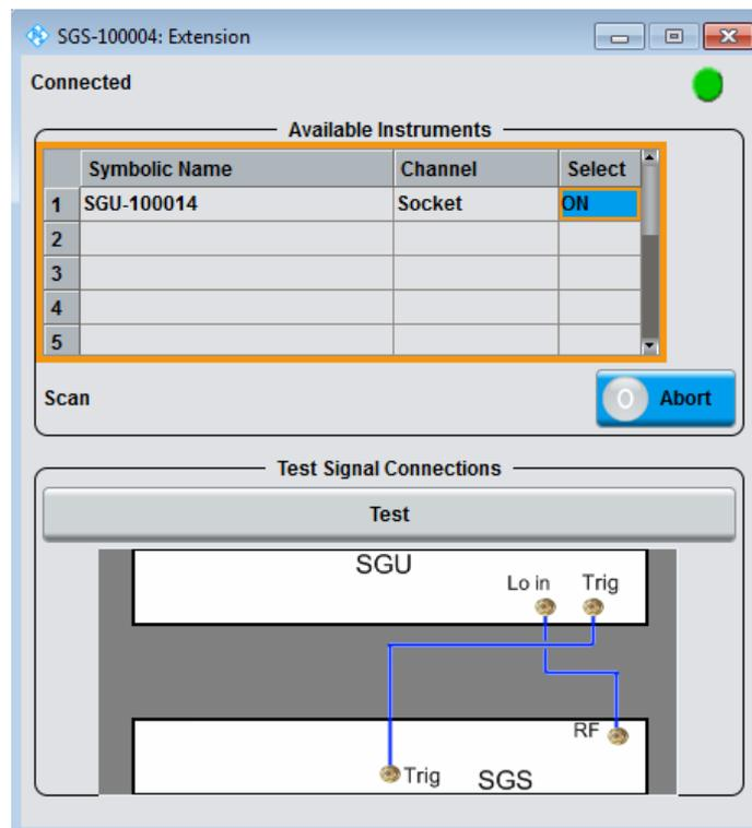
The diagram displays the connection state of the tested connections.
