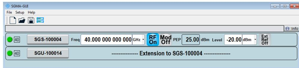
The extension adopts these values and states automatically. Also, it generates a CW signal with RF = 40 GHz and Level = -20 dBm.
