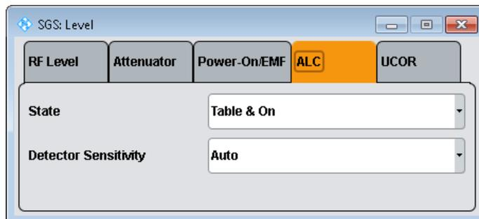
You can use automatic level control (ALC) with almost all applications, especially I/Q modulation. Deactivate ALC for certain settings in the baseband and when I/Q impairments are active ("Impairments > On").
