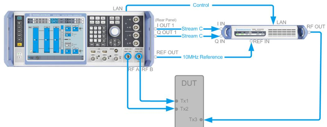
Figure 7-3: Configuration example: Control from an R&S SMW
