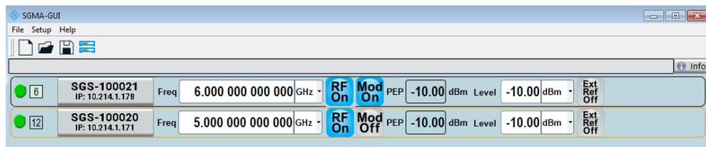
The 5 GHz signal is output at the "RF 50Ω" connector at the rear panel of the R&S SGS.
