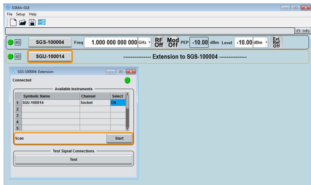
9. Select "Test Signal Connections > Test" to trigger a check of all required signal connections.
