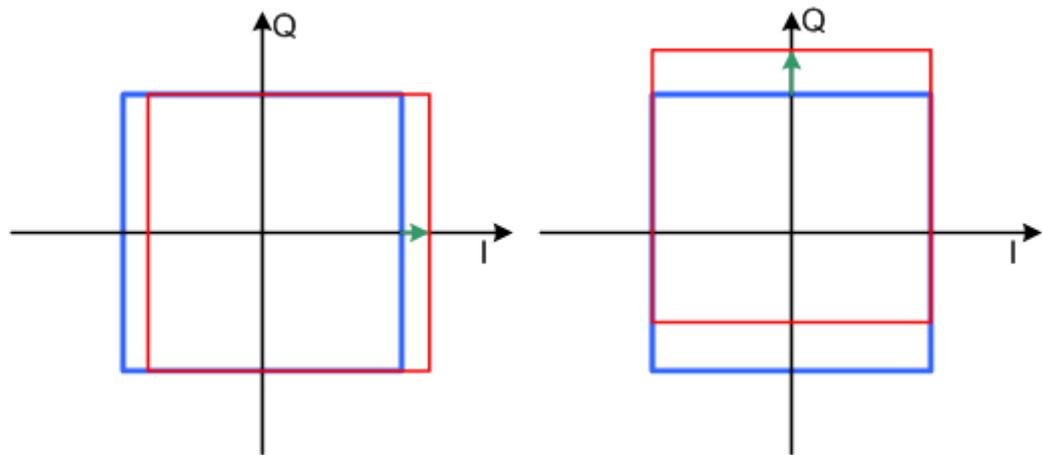
Figure 9-8: I offset (left) and Q offset (right) in the I/Q constellation diagram
