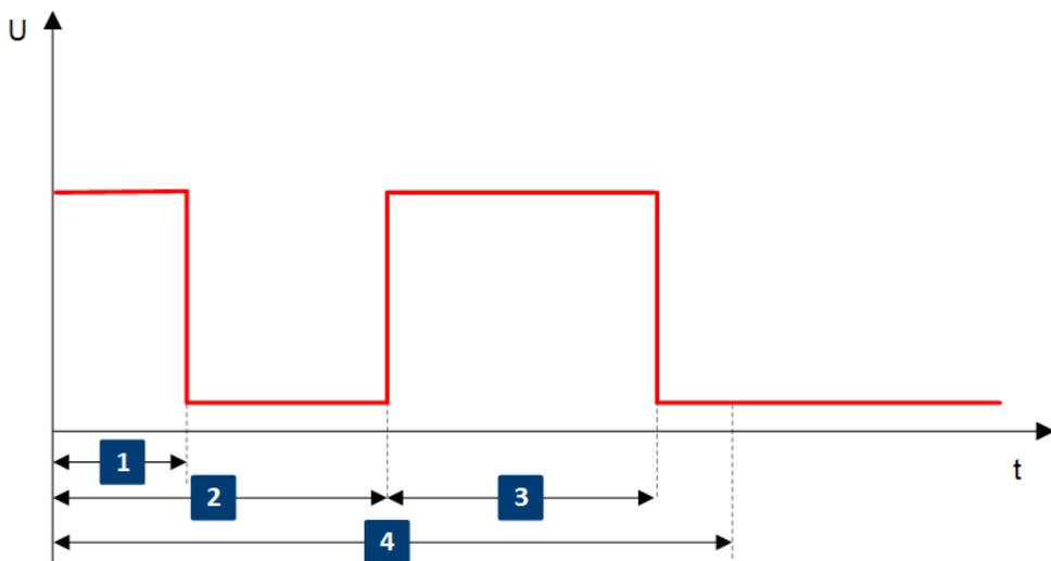
Figure 9-5: Pulse generator - double pulse mode
