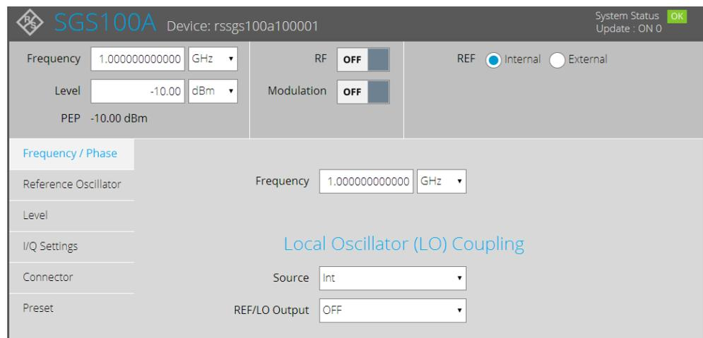
In the R&S SGS100A Web-GUI main panel, the green indicator "System Status > OK " confirms that there is a connection between the instrument and the remote PC and that the instrument is recognized by the software.
