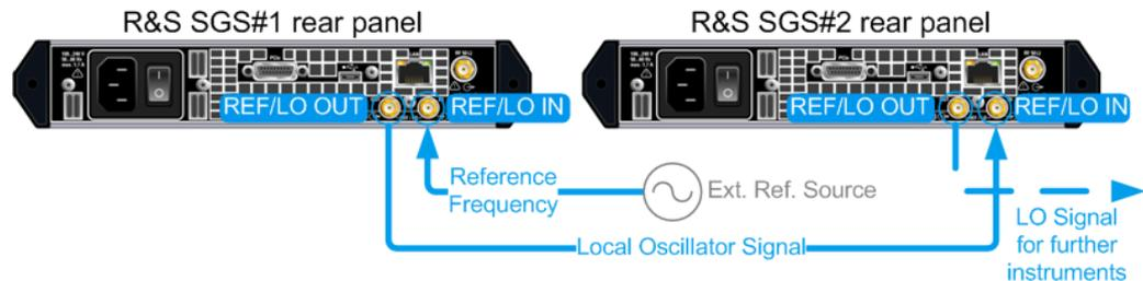
*Figure 11-3: Example of a setup: LO coupling*
