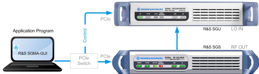
Figure 7-7: Connection of an R&S SGS and an R&S SGU through a PCIe switch
