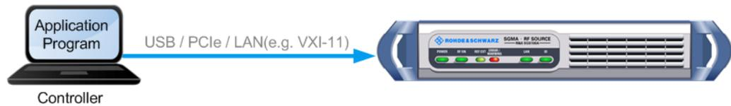
Figure 7-2: Configuration example: remote control from a controller
