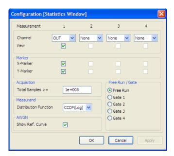
Figure 5-56: Measure > Statistics > Meas configuration
