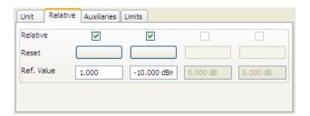
Figure 5-81: Measure > Numerical > Math configuration > Relative
