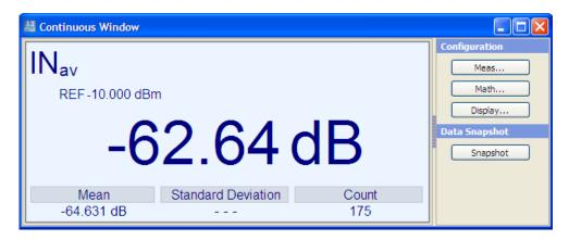
Figure 3-2: Numeric measurement window of R&S NRPV
