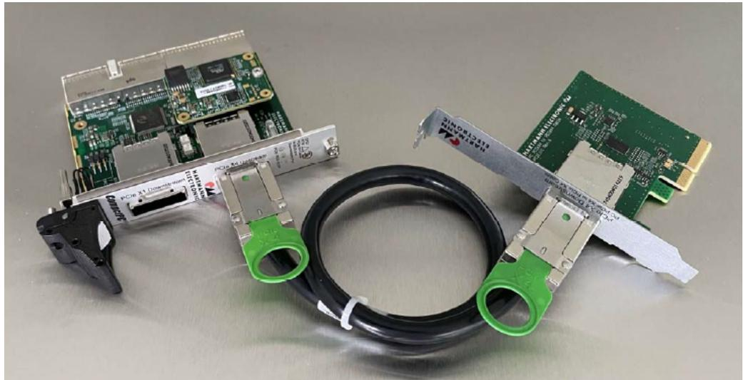
*Figure 11-27: Cabling of the R&S TS-PSC08x components.*
