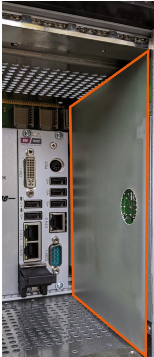
*Figure 3-3: Install insulation plate (1152.3443.00)*
