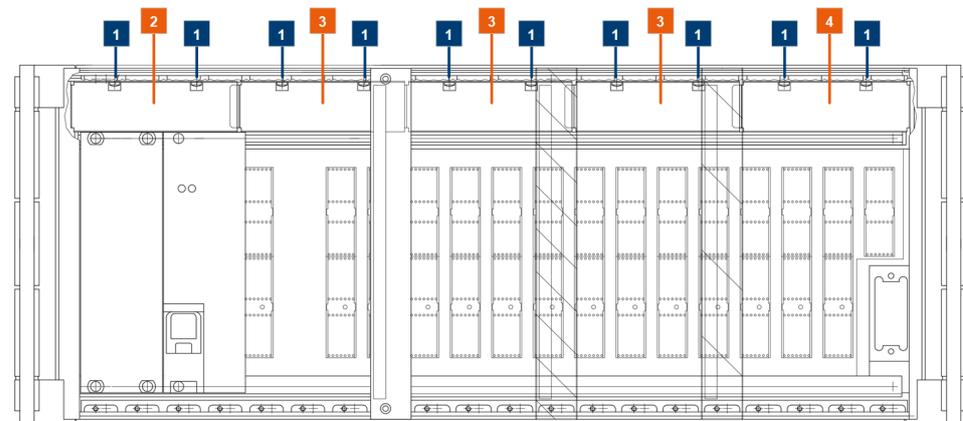
**Figure 8-2: Mount shielding kit covers (front view)**
