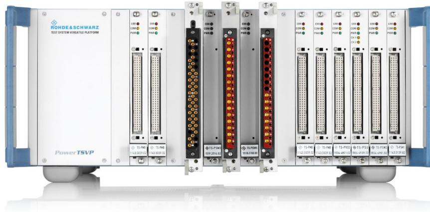
The R&S PowerTSVP chassis is a cost-efficient subsystem for high-power and switching applications. It can be used to build systems ranging from dedicated switching instruments to more complex switching applications in test and measurement systems. The chassis contains a mechanical frame, digital backplane, analog measurement bus, mains switching and filtering, power supply and diagnostic extensions, controlled via CAN bus.
