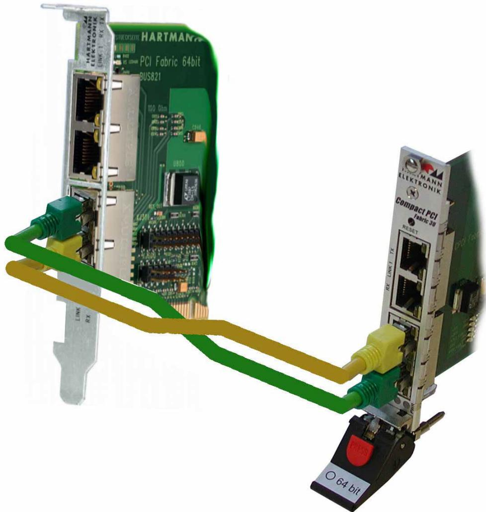
**Figure 11-25: Cabling of the R&S TS-PSC0 components.**
