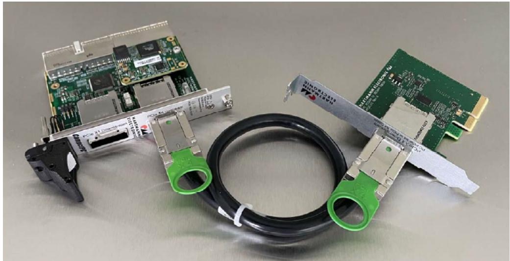
Figure 3-6: Cabling of the R&S TS-PSC08 components.
