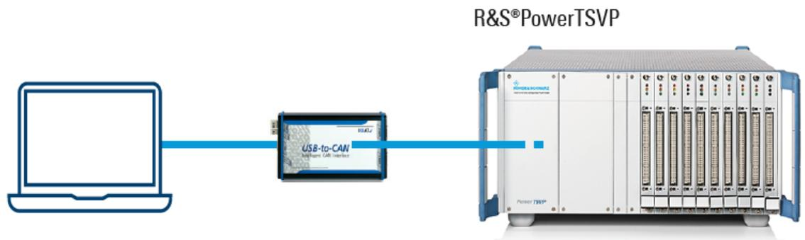
Figure 3-7: R&S PowerTSVP to external PC connection
