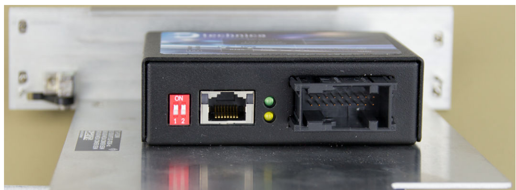
Figure 5-3: R&S TS-PSCBRR BroadR-Reach Media Converter 100Base-T1 BCM internal connectors
