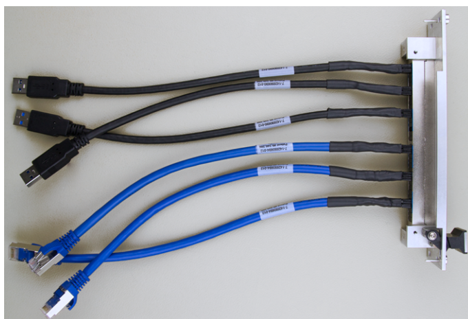
Figure 4-3: Side view of R&S TS-PFP9 VTAC Interface Front Panel
