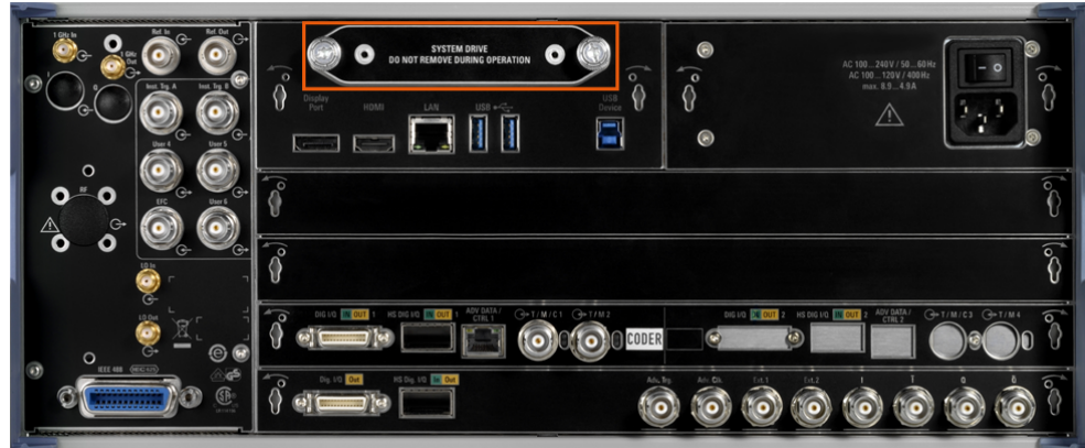
Figure 5-1: Location of the hard disk drive
