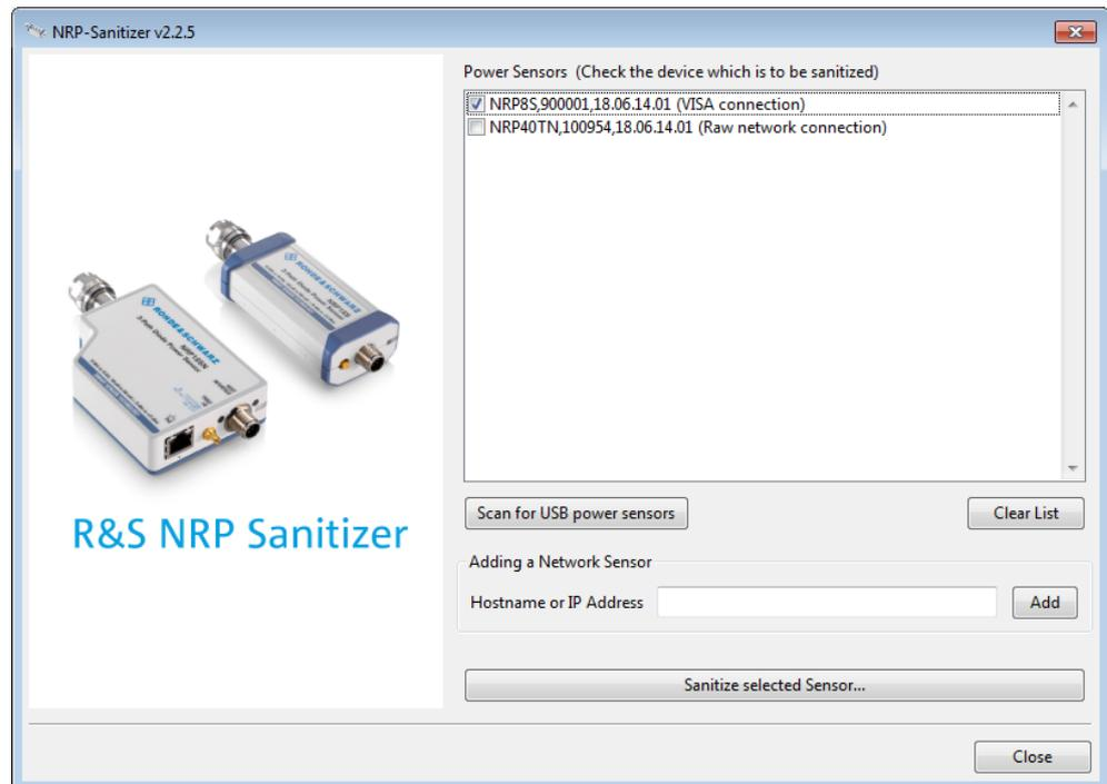
The R&S NRP Sanitizer tool scans automatically for USB power sensors. For LAN power sensors, enter the corresponding address information in the "Hostname or IP Address" field to add the sensor to the list.
