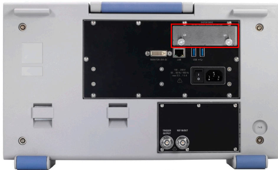
Figure 5-1: Location of the R&S RTE HDD/SSD
