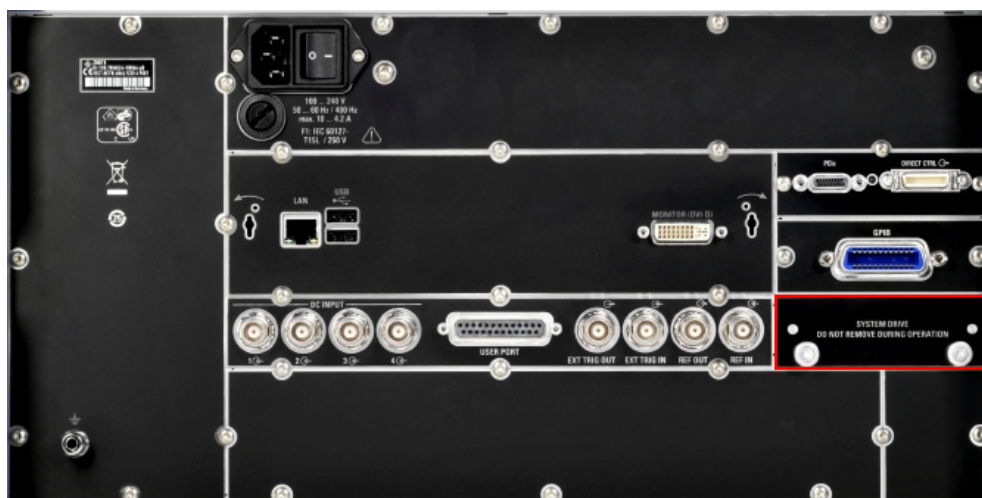
Figure 5-1: Location of the system drive for R&S ZNB (1st gen), R&S ZNBT, and R&S ZNC
