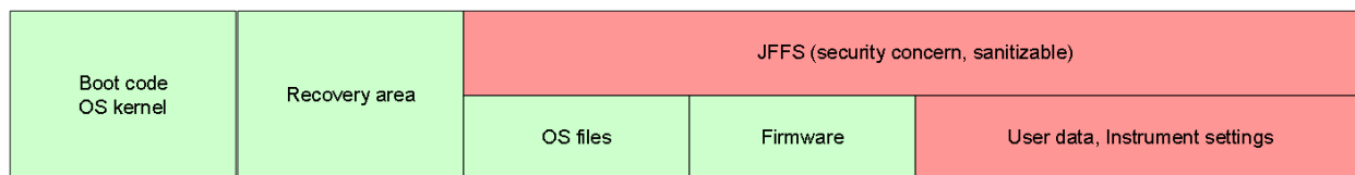
Figure 4-1: Logical sections of the Flash memory
