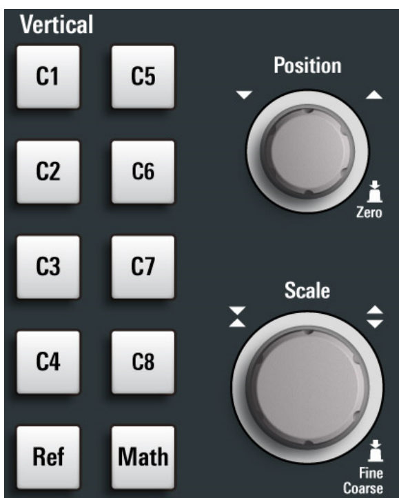
Figure 5-5: Vertical controls of MXO 5 with 8 input channels
