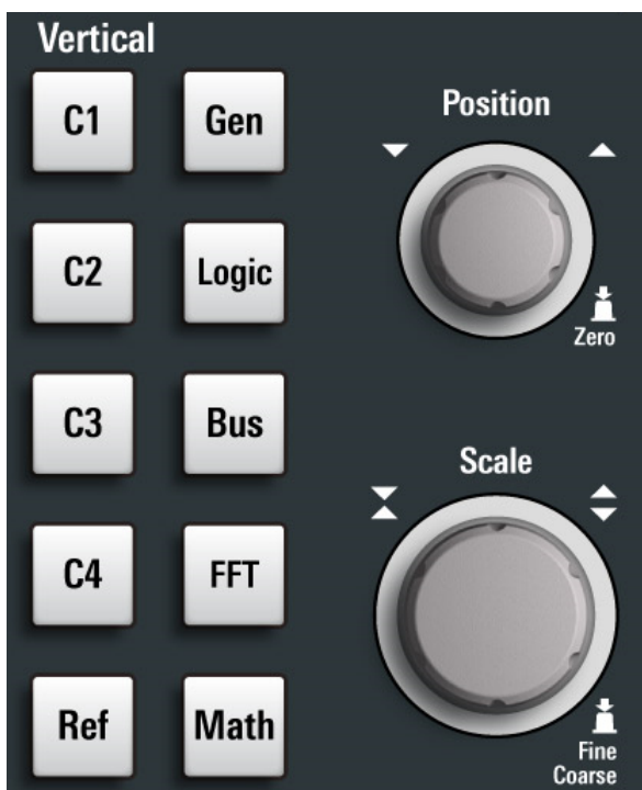
Figure 5-4: Vertical controls of MXO 5 with 4 input channels
